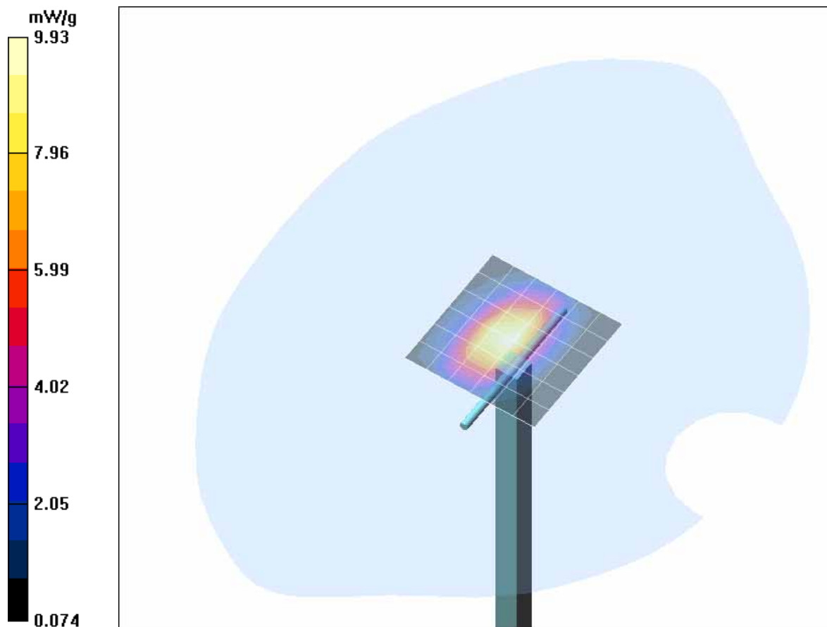
Fig. 10: Validation measurement 1900 MHz Head (August 29, 2005), coarse grid. Ambient Temperature: 22.5°C, Liquid Temperature: 21.3°C.
