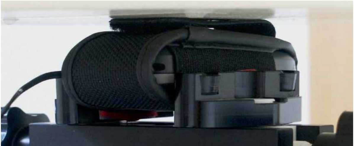
Fig. 25: Body worn configuration, GSM with headset and FCT650, antenna towards the phantom (10 mm distance).
