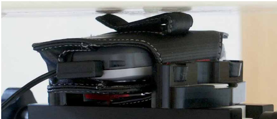
Fig. 26: Body worn configuration, GSM with headset and FCL600, antenna towards the phantom (13 mm distance).
