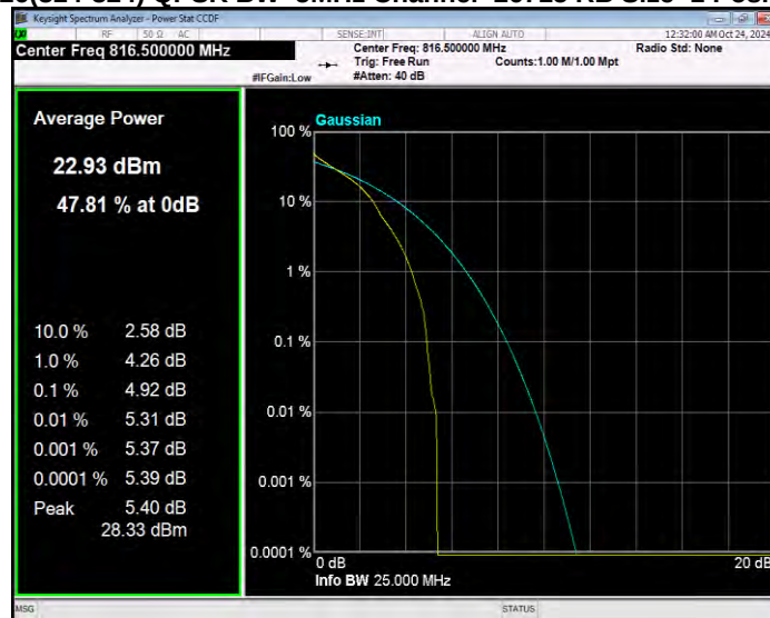
Band26(814-824) QPSK BW=5MHz Channel=26740 RB Size=1 Position=#0
