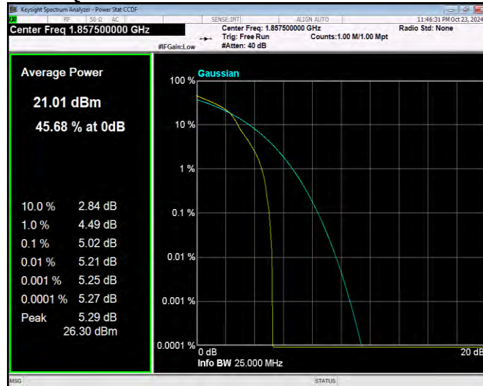
Band25 16QAM BW=15MHz Channel=26115 RB Size=1 Position=#0
