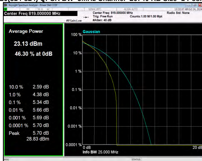
Band26(814-824) QPSK BW=5MHz Channel=26740 RB Size=1 Position=#0
