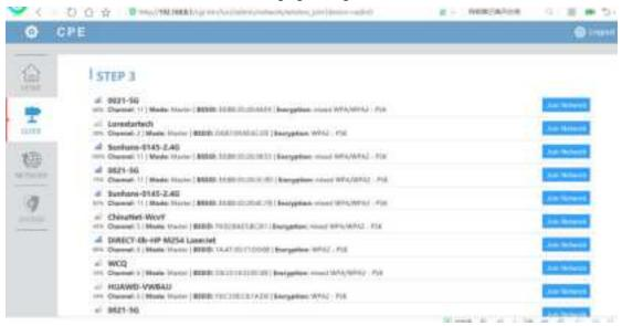
After the bridge is successfully connected, the main AP can perform point-to-point WiFi signal transmission with the Station AP
