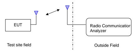
This configuration is Radiated emission measurement
