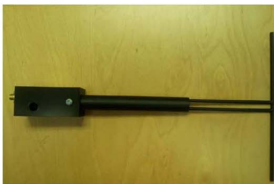
Figure 1 – MVG COMOSAR Validation Dipole
