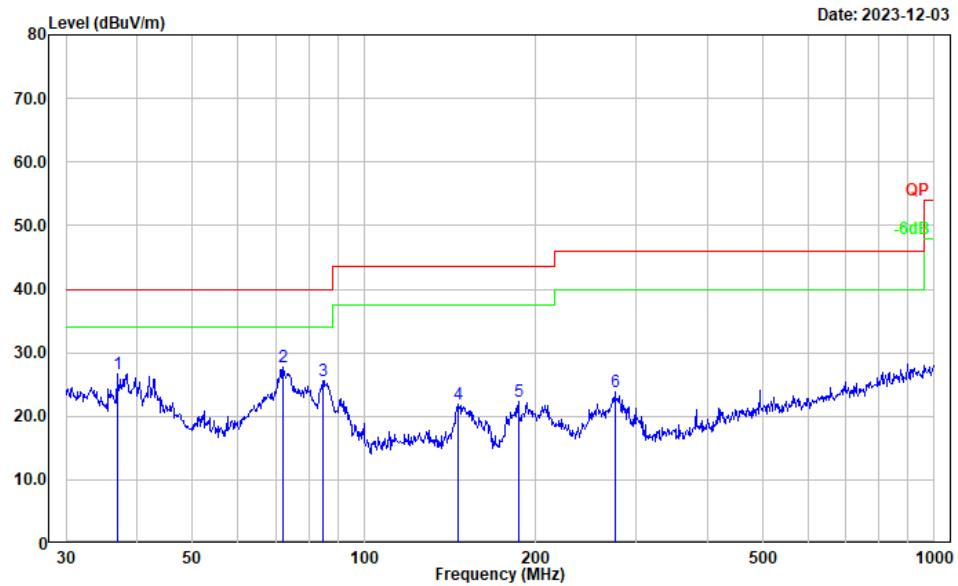
**Frequency Band 5725-5850 MHz:***(Tested at maximum output power mode: 802.11a mode)***802.11a \_ Low Channel \_ Horizontal**
