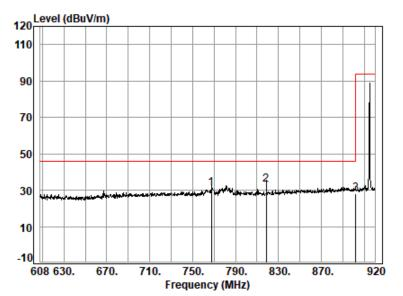
Site : chamber Condition: 3m HORIZONTAL Job No. : 02309AT/02310AT Test mode: 00 : 6\*14 Sample 1 Ant Cable Preamp Limit 0ver Read Freq Factor Loss Factor Limit Remark Level Level Line MHz dB/m dB dB dBuV dBuV/m dBuV/m dB 1 767.74 26.65 3.73 27.71 28.16 30.83 46.00 -15.17 QP 2 q 818.91 26.98 3.88 27.52 29.90 33.24 46.00 -12.76 QP 3 902.00 28.67 4.10 27.12 22.53 28.18 46.00 -17.82 QP
