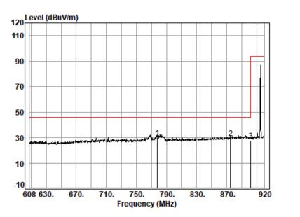
Site : chamber Condition: 3m HORIZONTAL : 02309AT/02310AT Job No. Test mode: 00 : 8\*8 Sample 1 Ant Cable Preamp 0ver Read Limit Loss Factor Level Level Line Limit Remark Freq Factor dBuV dBuV/m dBuV/m MHz dB/m dB dB dB 27.19 30.02 46.00 -15.98 QP 1 q 778.04 26.75 3.76 27.68 2 875.38 28.21 4.03 27.25 24.76 29.75 46.00 -16.25 QP 28.67 4.10 27.12 21.84 27.49 46.00 -18.51 QP 3 902.00
