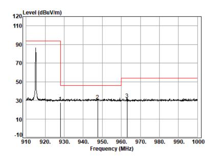
Site : chamber Condition: 3m HORIZONTAL Job No. : 02309AT/02310AT Test mode: 00 : 8\*8 Sample 1 Ant Cable Preamp Read Limit 0ver Loss Factor Level Level Line Limit Remark Freq Factor dBuV dBuV/m dBuV/m MHz dB/m dB dB dB 28.43 4.16 27.00 21.98 27.57 46.00 -18.43 QP 1 928.00 2 q 4.21 26.90 947.62 28.70 23.69 29.70 46.00 -16.30 QP 3 963.01 28.38 4.25 26.83 25.39 31.19 54.00 -22.81 QP
