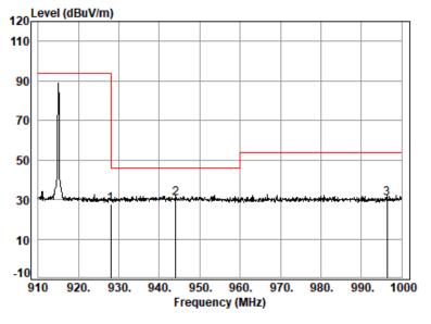
Site : chamber Condition: 3m HORIZONTAL Job No. : 02309AT/02310AT Test mode: 00 : 6\*14 Sample 1 Ant Cable Preamp 0ver Read Limit Freq Factor Loss Factor Level Level Line Limit Remark dBuV dBuV/m dBuV/m MHz dB/m dB dB dB 1 928.00 28.43 4.16 27.00 22.17 27.76 46.00 -18.24 QP 2 q 944.11 28.69 4.20 26.92 24.32 30.29 46.00 -15.71 QP 4.34 26.67 24.36 30.60 54.00 -23.40 QP 996.40 28.57 3
