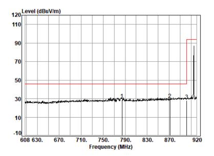
: chamber Site Condition: 3m VERTICAL : 02309AT/02310AT Job No. Test mode: 00 : 8\*8 Sample 1 Ant Cable Preamp Limit **Over** Read Freq Factor Loss Factor Level Level Line Limit Remark dBuV dBuV/m dBuV/m MHz dB dB/m dB dB 784.28 26.88 3.78 27.66 26.02 29.02 46.00 -16.98 QP 1 q 4.02 27.27 24.14 28.92 46.00 -17.08 QP 2 871.64 28.03 902.00 28.67 4.10 27.12 22.45 28.10 46.00 -17.90 QP 3
