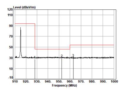
Site : chamber Condition: 3m VERTICAL Job No. : 02309AT/02310AT Test mode: 00 : 8\*8 Sample 1 Ant Cable Preamp **Over** Read Limit Freq Factor Loss Factor Level Level Line Limit Remark MHz dBuV dBuV/m dBuV/m dB/m dB dB dB 1 928.00 28.43 4.16 27.00 21.54 27.13 46.00 -18.87 QP 2 q 952.48 28.66 4.23 26.88 23.72 29.73 46.00 -16.27 QP 963.01 28.38 4.25 26.83 24.95 30.75 54.00 -23.25 QP 3
