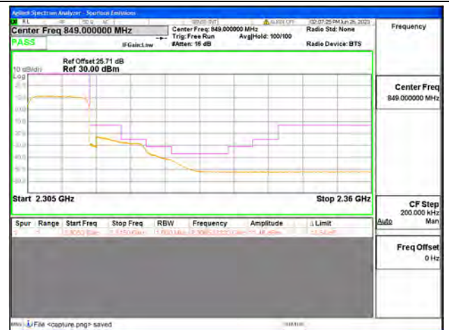
Band30 / 10MHz / High CH / QPSK / FULL RB
