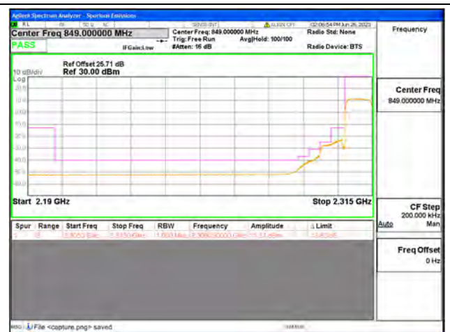
Band30 / 10MHz / Low CH / QPSK / FULL RB
