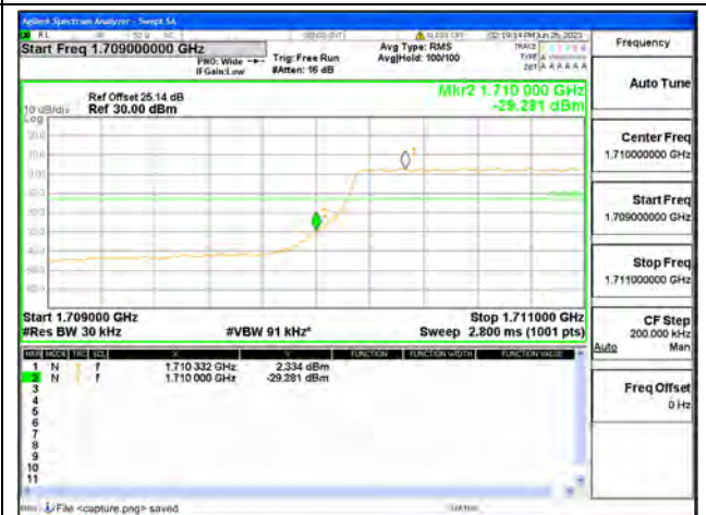
Band66 / 3MHz / Low CH / QPSK / FULL RB
