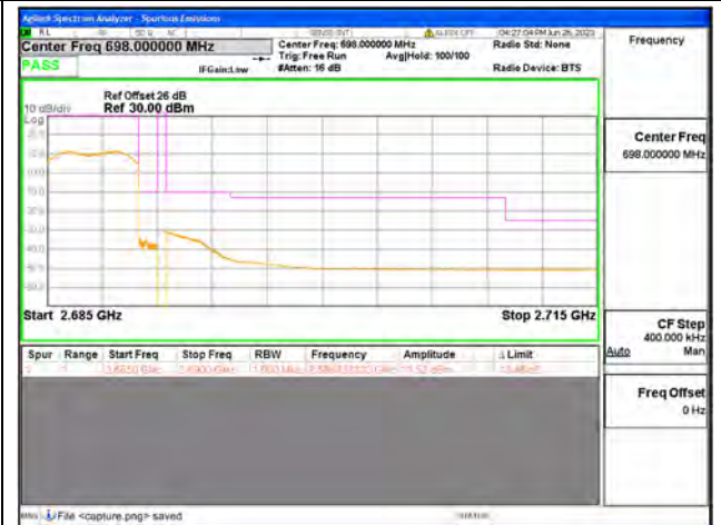
Band41 / 5MHz / High CH / QPSK / FULL RB
