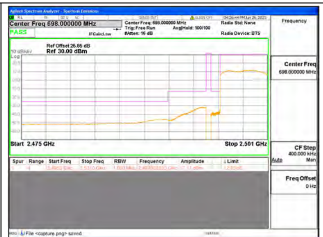
Band41 / 5MHz / Low CH / QPSK / FULL RB
