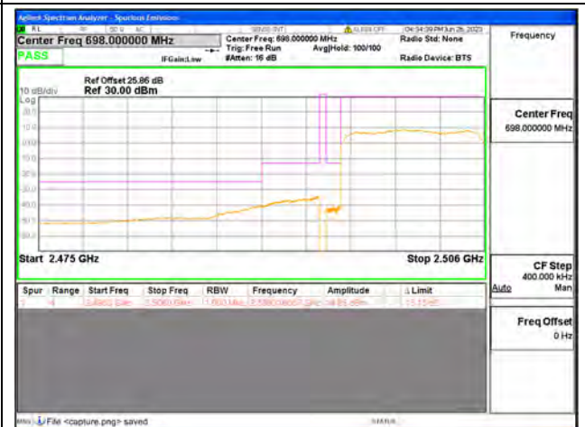
Band41 / 10MHz / Low CH / QPSK / FULL RB
