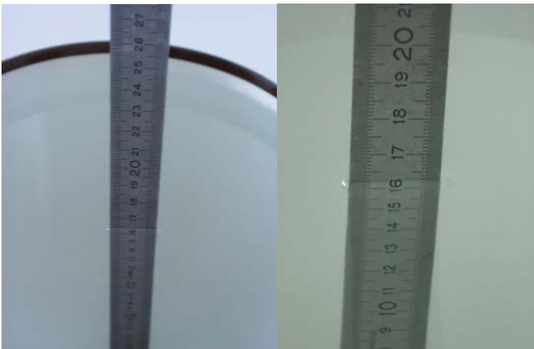
Fig. 23: Liquid depth for PCS 1900 Head and Body measurements.
