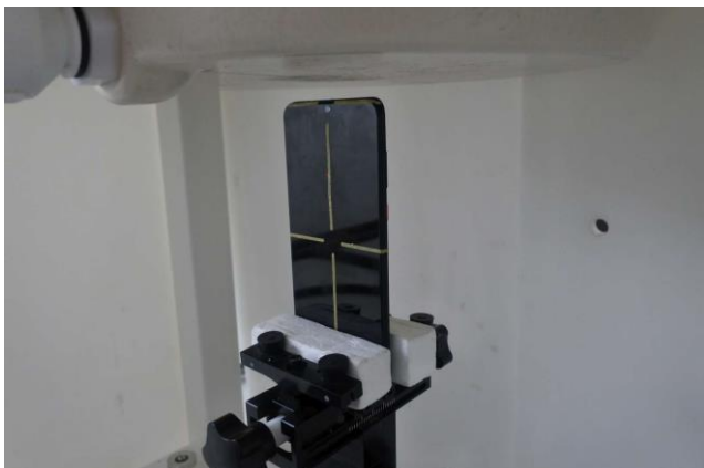
Top Side, Test Separation 10 mm
