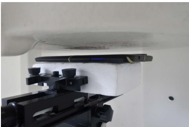
Back, Test Separation 10 mm
