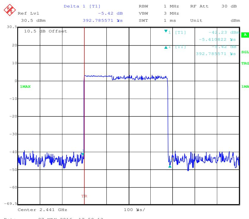
**Pulse time, High Channel, 3DH1**
