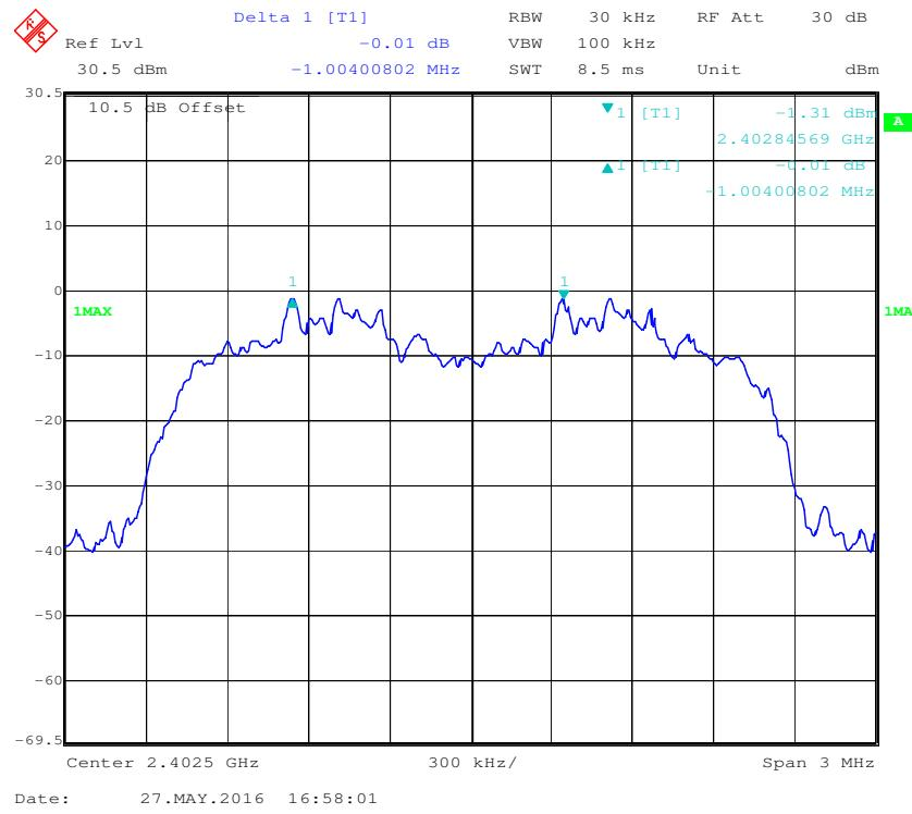
**EDR (8DPSK): Middle Channel**
