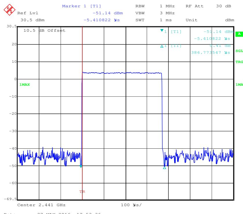
**Pulse time, High Channel, DH1**
