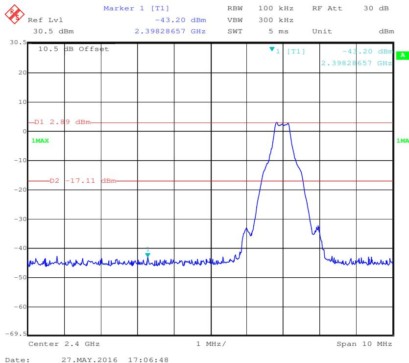
**BDR (GFSK): Band Edge-Right Side**
