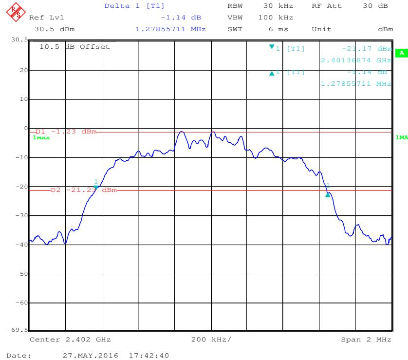
**EDR (8DPSK): Middle Channel**
