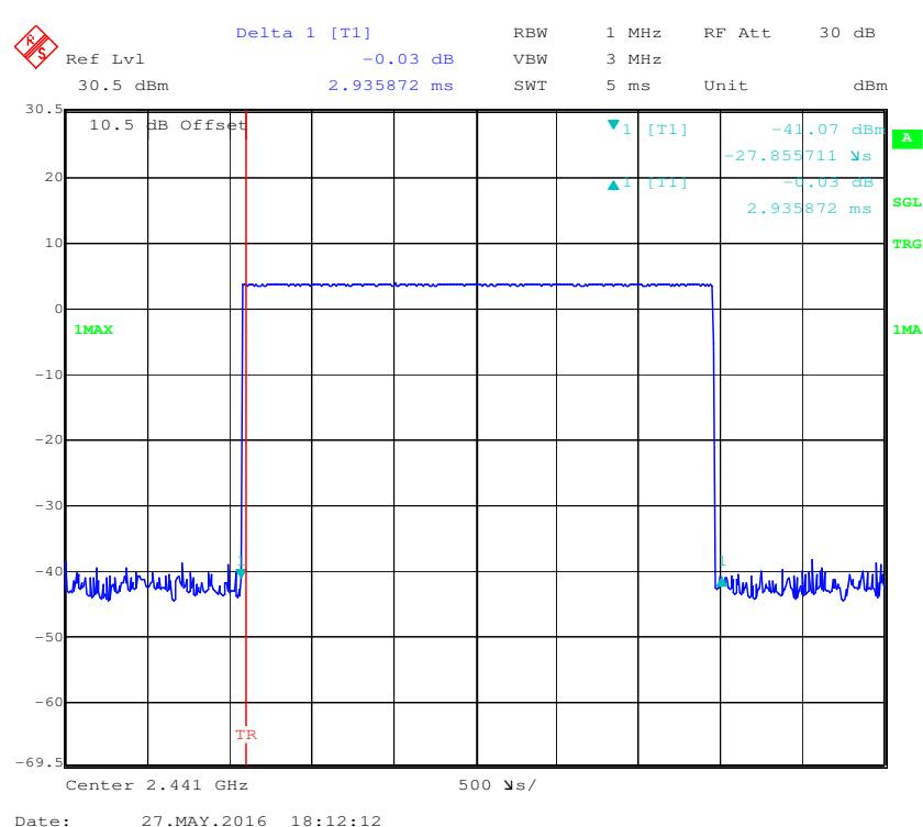
**Pulse time, High Channel, DH5**
