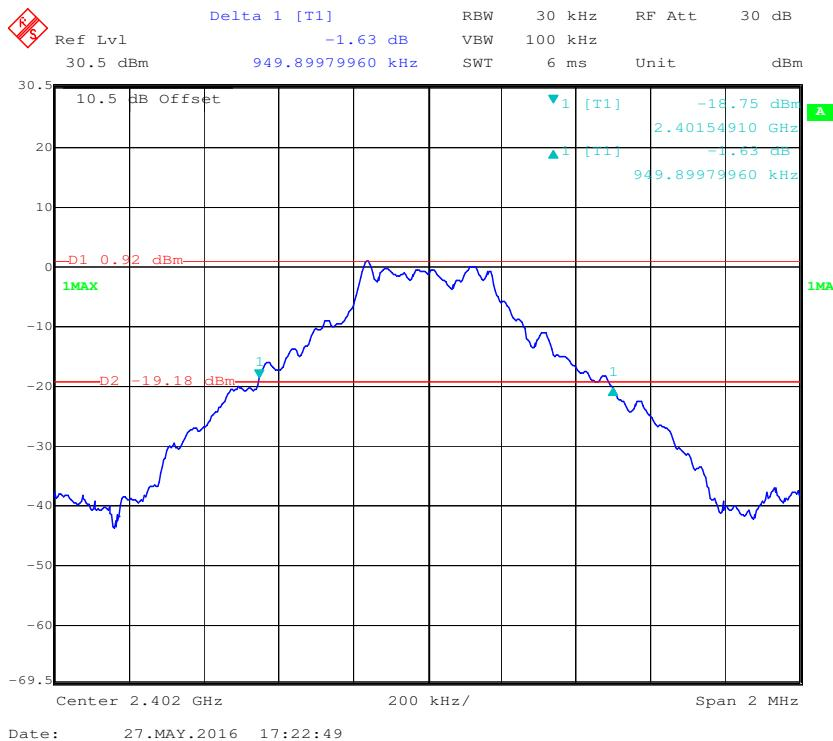
**BDR (GFSK): Middle Channel**
