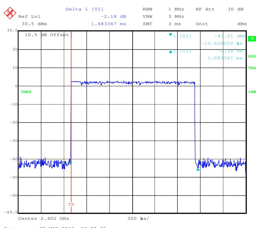
**Pulse time, Middle Channel, 3DH3**
