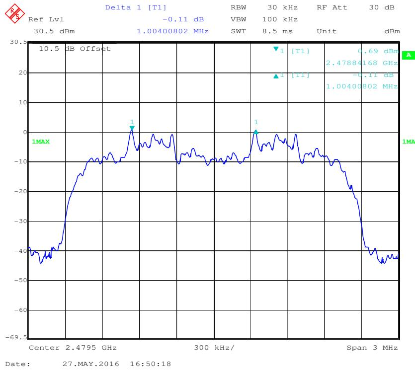
**EDR (8DPSK): Low Channel**
