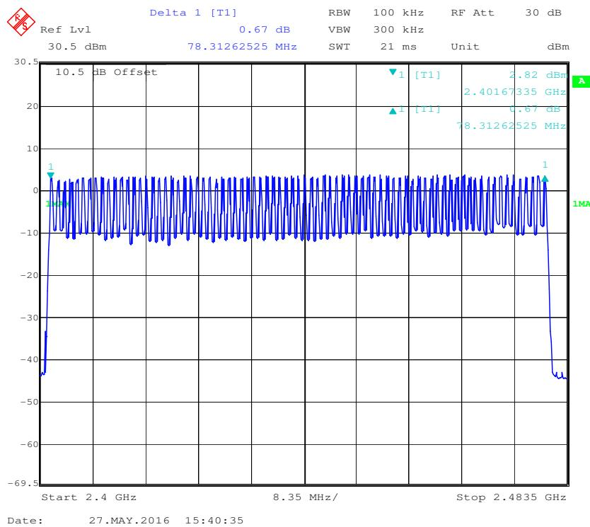
**EDR ( $\pi/4$ -DQPSK): Number of Hopping Channels**
