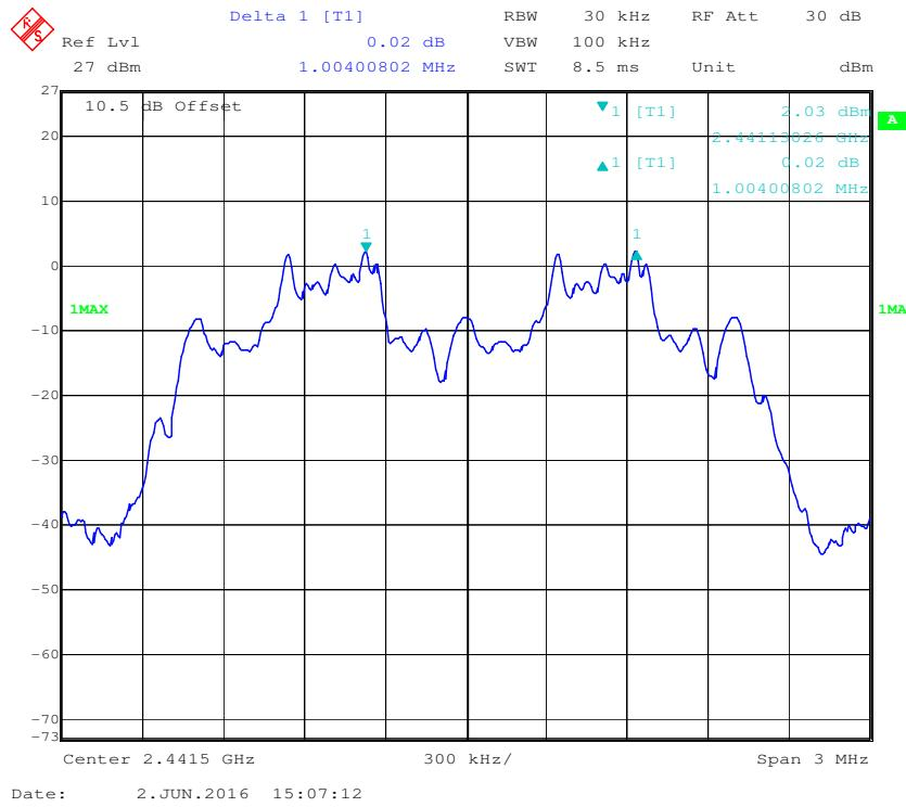
**EDR ( $\pi/4$ -DQPSK): High Channel**
