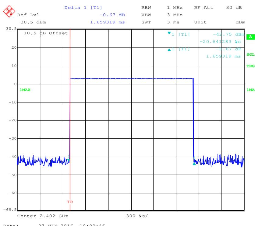
**Pulse time, Middle Channel, DH3**
