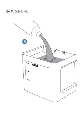
• After pouring into IPA, cover the inner lid. The IPA between 3L and the maximum fill line.
