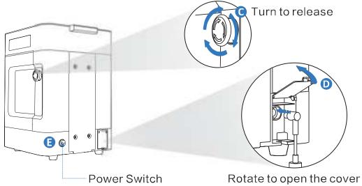
Press the power switch to turn it on. The outer lid opens, and the platform mount and basket raise in position.
