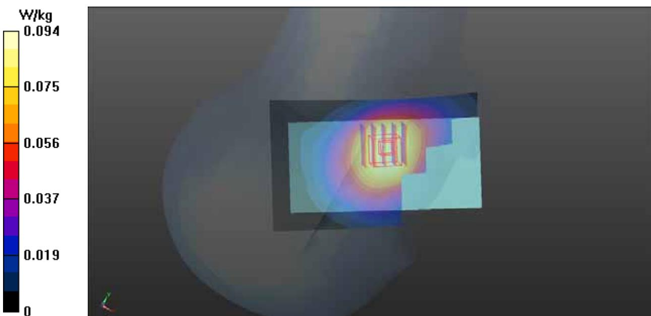
**P12 2.4G WLAN\_802.11b\_Left Cheek\_Ch6\_Sample2****DUT: 150324C20**
