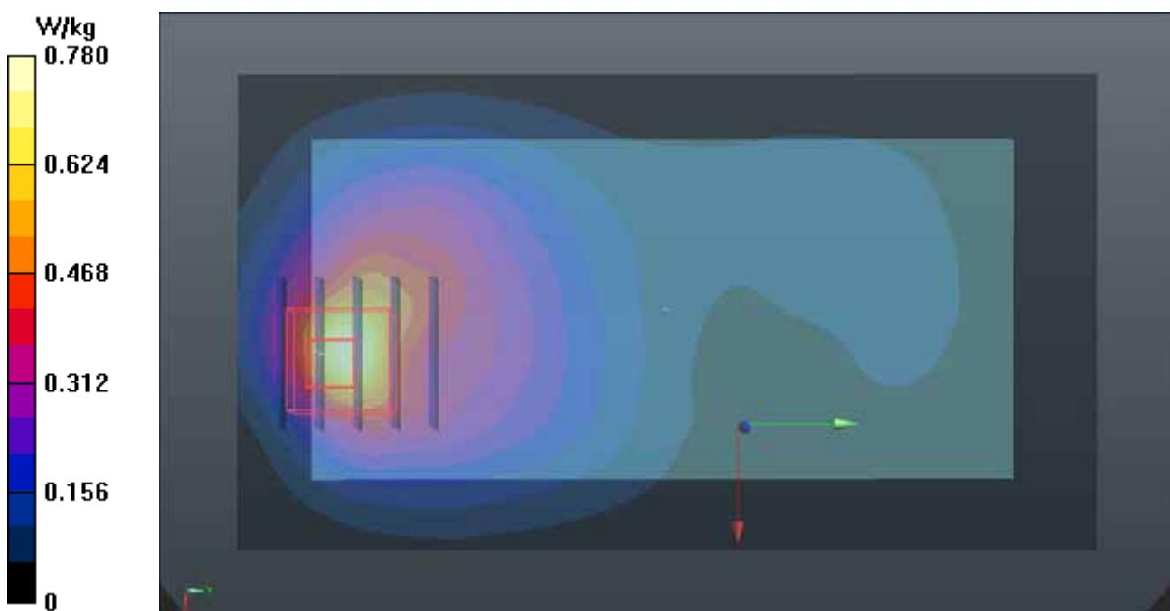
**P21 LTE 5\_QPSK10M\_Front Face\_1cm\_Ch20600\_Sample1\_1RB\_OS24****DUT: 150324C20**
