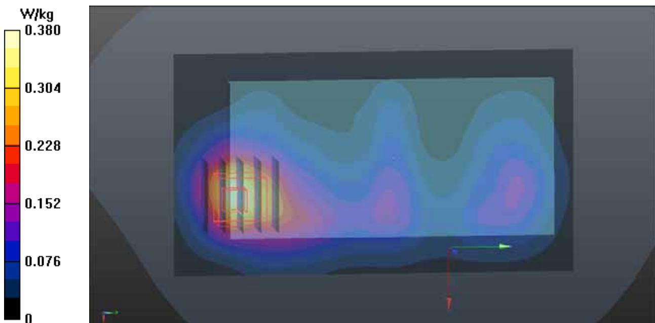
**P23 LTE 13\_QPSK10M\_Front Face\_1cm\_Ch23230\_Sample1\_1RB\_OS0****DUT: 150324C20**
