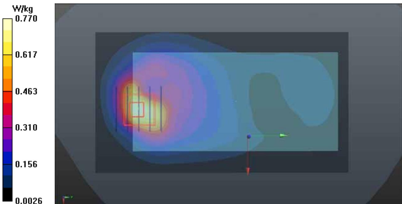
**P20 LTE 4\_QPSK20M\_Rear Face\_1cm\_Ch20175\_Sample1\_1RB\_OS0****DUT: 150324C20**
