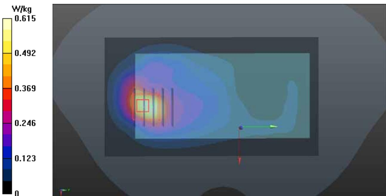
**P19 LTE 2\_QPSK20M\_Rear Face\_1cm\_Ch18700\_Sample2\_1RB\_OS0****DUT: 150324C20**
