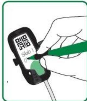
**3** Assign the sensor a name in the mobile app and on its label
