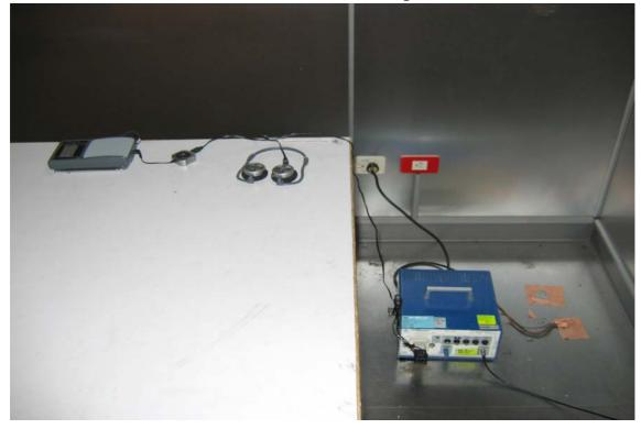
**Conducted Emission Set up Photo**
