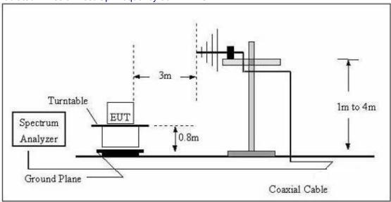
(C) Radiated Emission Test-Up Frequency Above 1GHz
