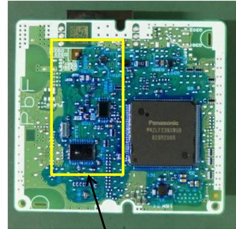
125kHz transmission circuit
