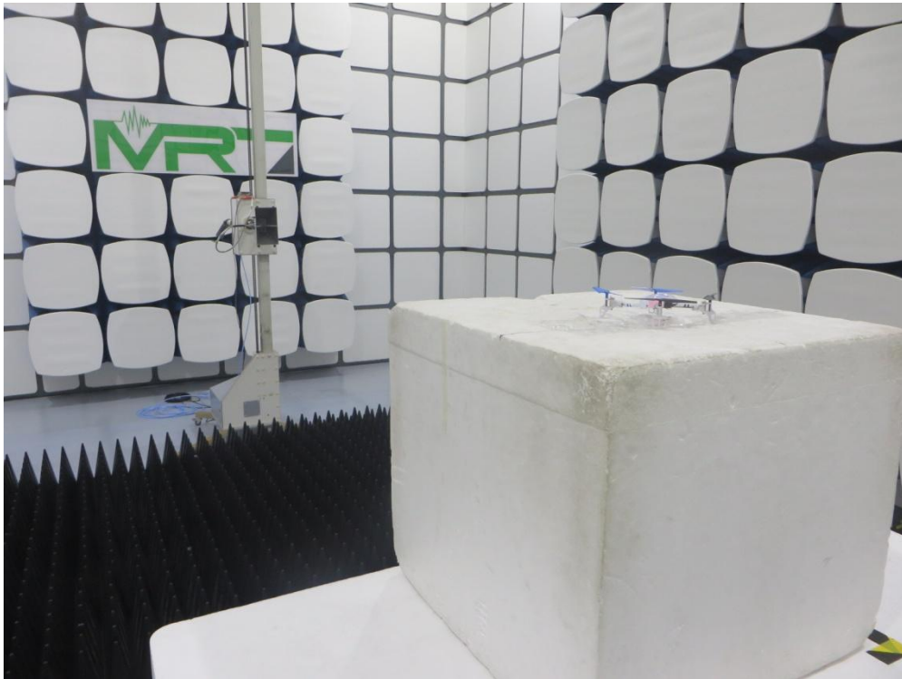
Description: Radiated Spurious Emissions Test Setup for 1GHz ~ 18GHz
