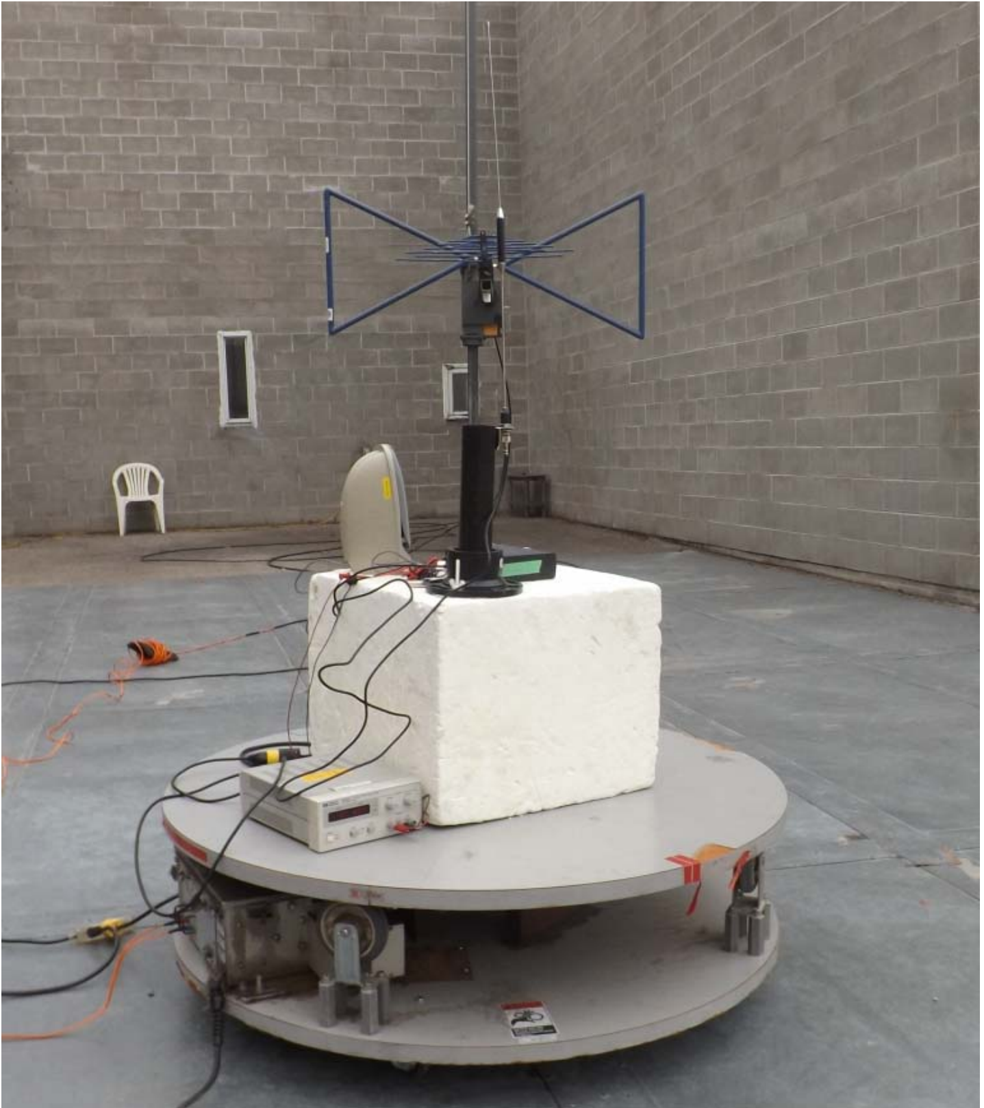
Figure E23.12 – Setup, RE Rx (DXX) Above 30MHz, with Accessories
