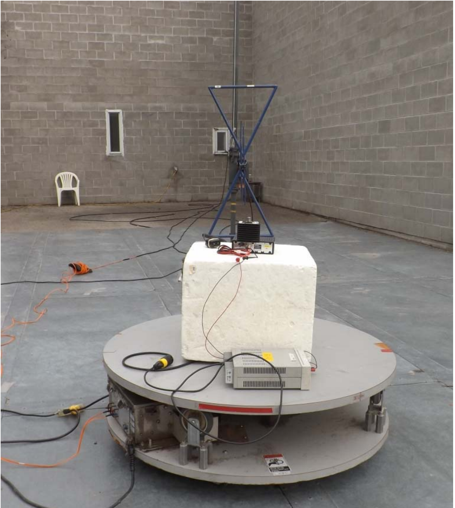
Figure E23.3 – Setup, Above 30MHz, without Accessories
