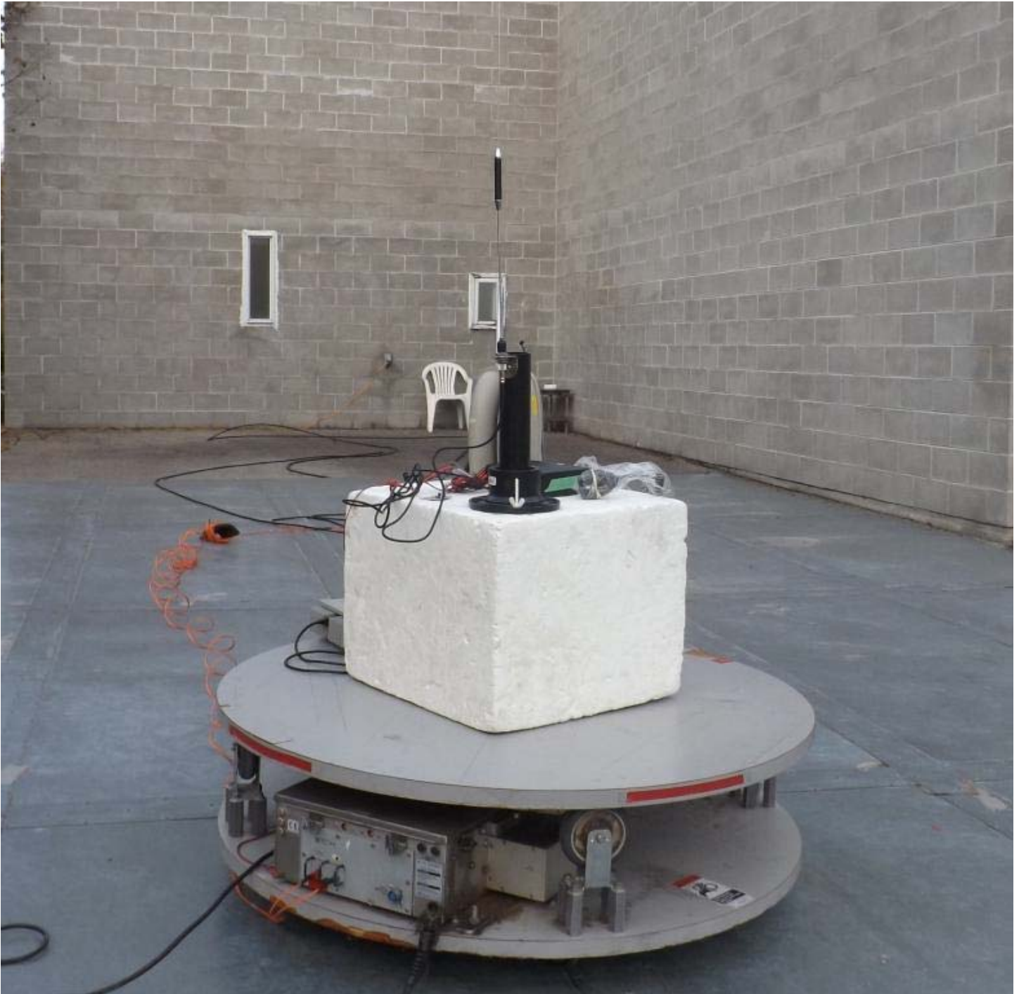
Figure E23.2 – Setup, Below 30MHz, with Accessories
