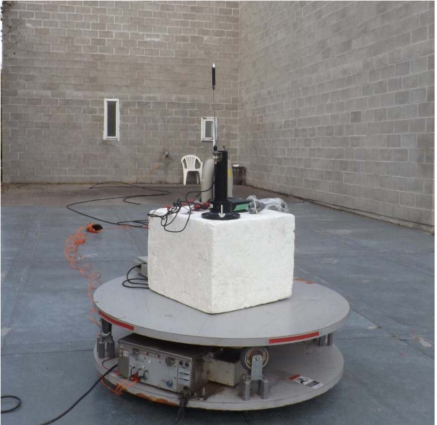
Figure E23.11 – Setup, RE Rx (DXX) Below 30MHz, with Accessories
