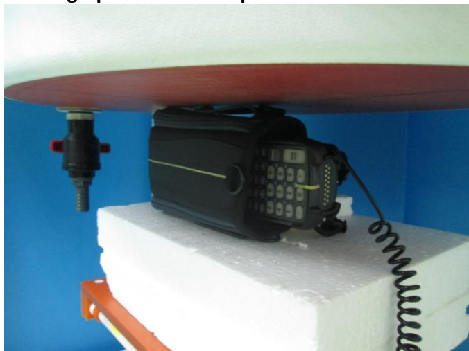
EUT + Holster 2 — Right Side with 0 cm Gap
