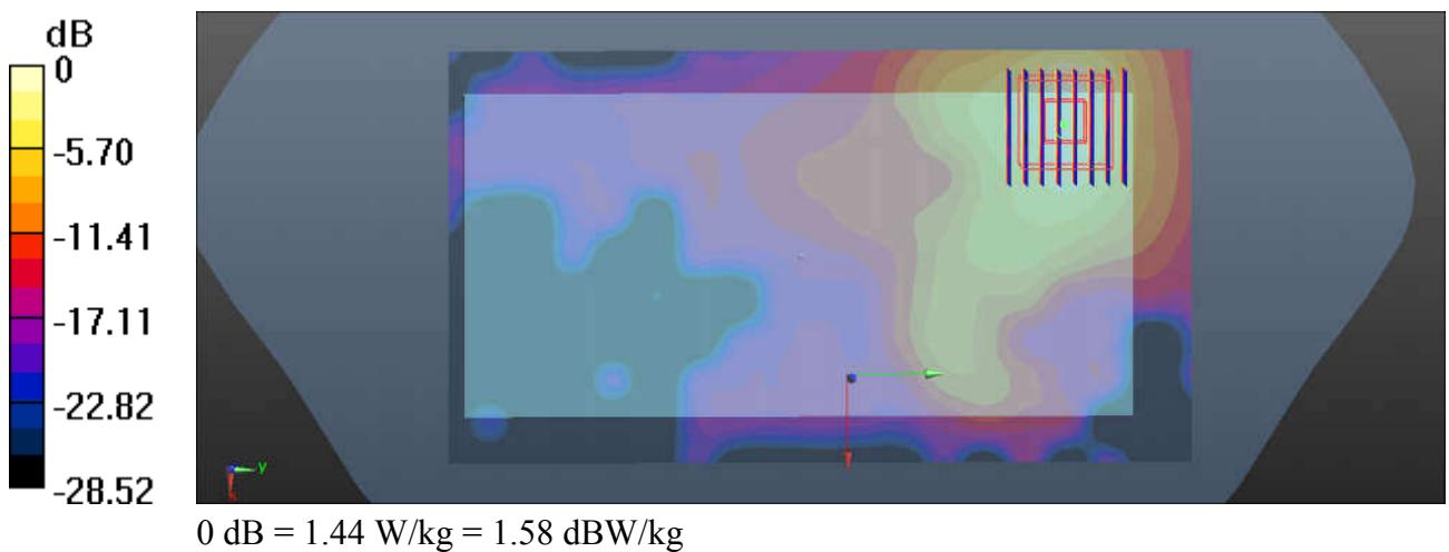
**70\_WLAN5.5GHz\_802.11n-HT20 MCS0\_Back\_10mm\_Ch100\_Ant 1+2**
