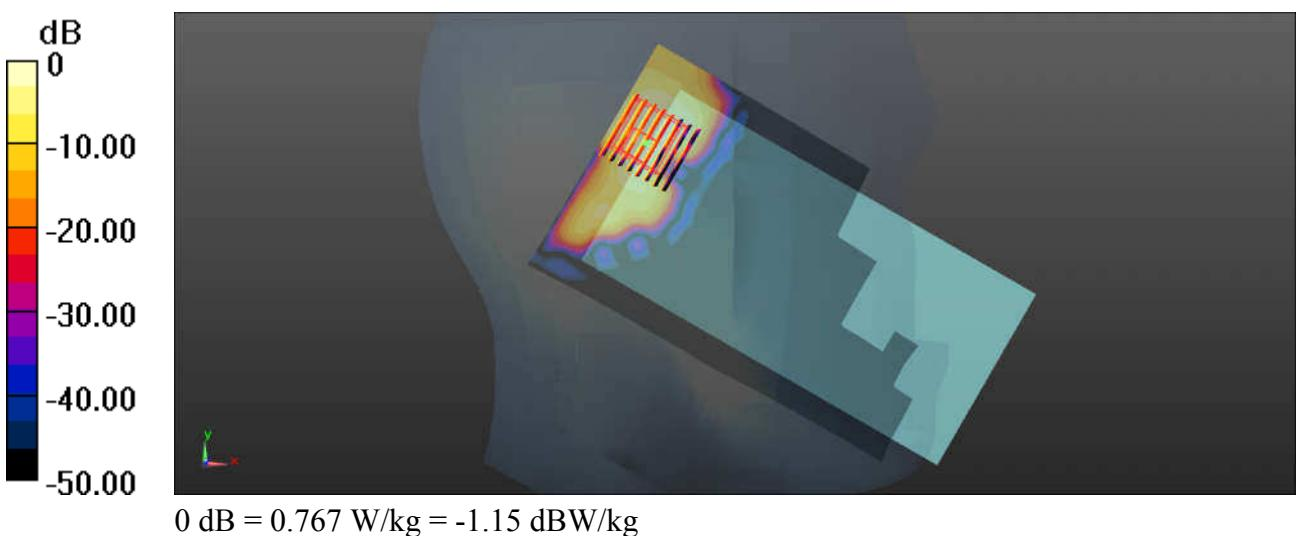
**25\_WLAN5.8GHz\_802.11a 6Mbps\_Left Cheek\_0mm\_Ch157\_Ant 1**
