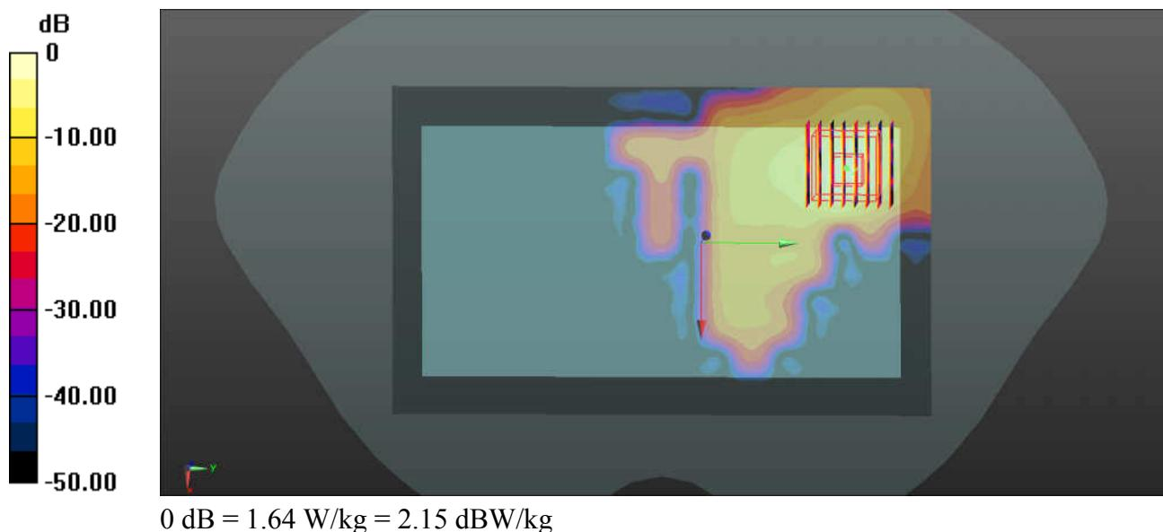
**48\_WLAN5GHz\_802.11a 6Mbps\_Back\_10mm\_Ch36\_Ant 2**
