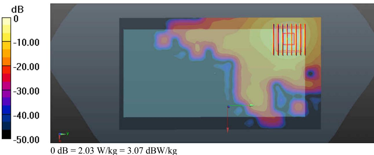
**50\_WLAN5.8GHz\_802.11a 6Mbps\_Back\_10mm\_Ch157\_Ant 1**
