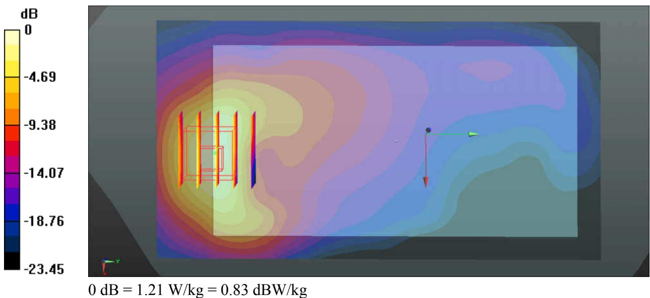
**61\_LTE Band 25\_20M\_QPSK\_1RB\_0Offset\_Back\_10mm\_Ch26140**
