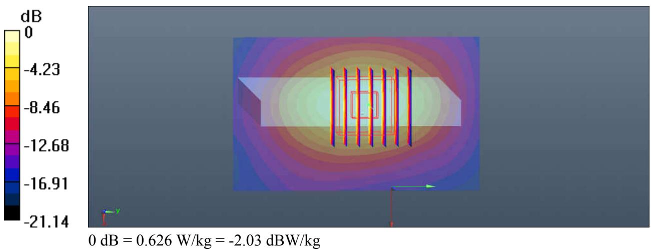
**47\_WLAN5.2GHz\_802.11a 6Mbps\_Back\_10mm\_Ch44\_Ant 1**
