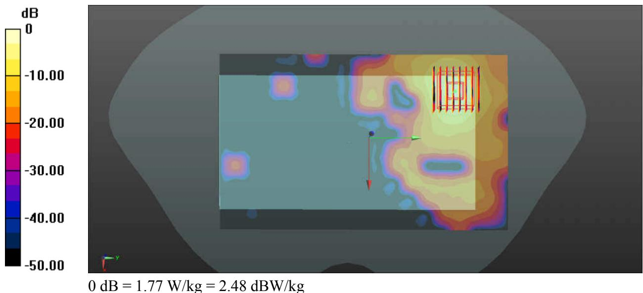
**49\_WLAN5.2GHz\_802.11n-HT20 MCS0\_Back\_10mm\_Ch36\_Ant 1+2**
