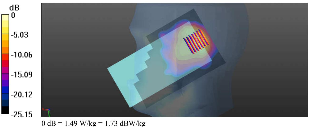
**19\_WLAN5.3GHz\_802.11a 6Mbps\_Left Cheek\_0mm\_Ch64\_Ant 1**
