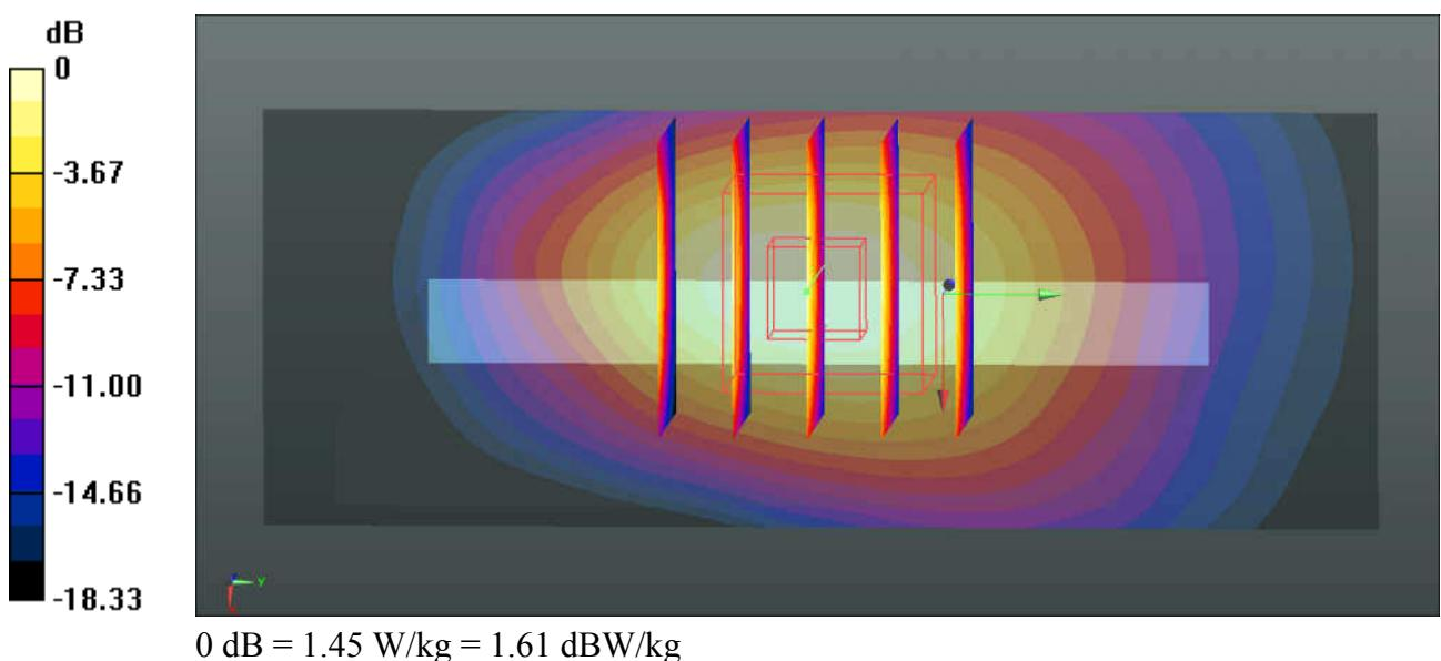
**36\_LTE Band 12\_10M\_QPSK\_1RB\_25Offset\_Right Side\_10mm\_Ch23095**
