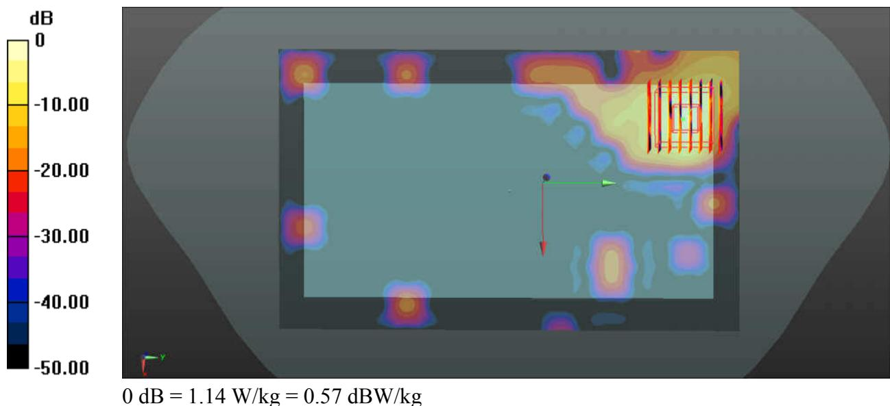
**69\_WLAN5.5GHz\_802.11n-HT20 MCS0\_Back\_10mm\_Ch140\_Ant 2**
