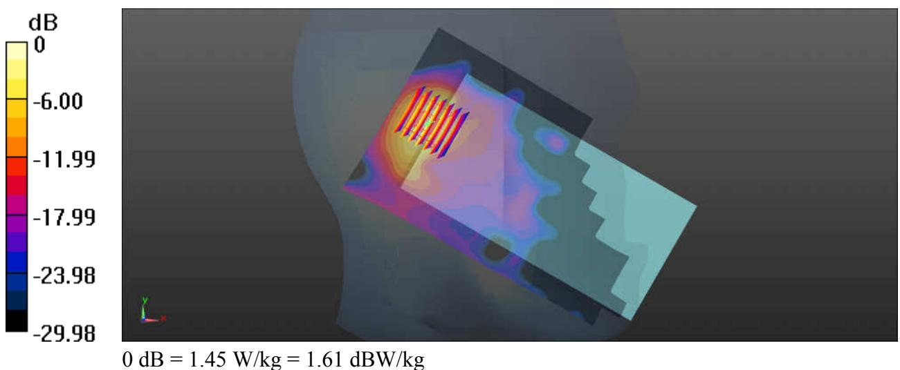
**18\_WLAN2.4GHz\_802.11n-HT20 MCS0\_Right Cheek\_0mm\_Ch11\_Ant1+2**
