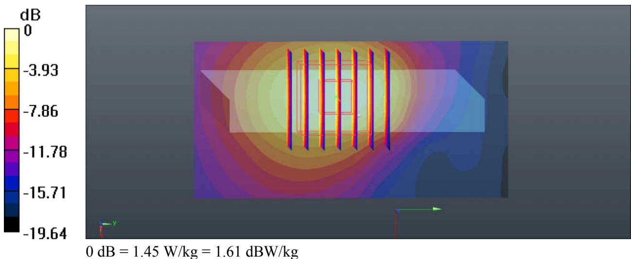
**45\_WLAN2.4GHz\_802.11b 1Mbps\_Top Side\_10mm\_Ch11\_Ant 2**
