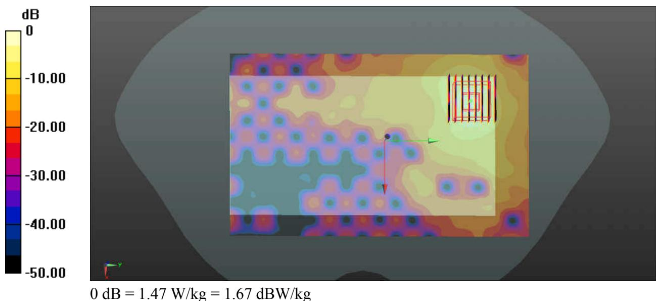
**67\_WLAN5.3GHz\_802.11n-HT20 MCS0\_Back\_10mm\_Ch52\_Ant 1+2**
