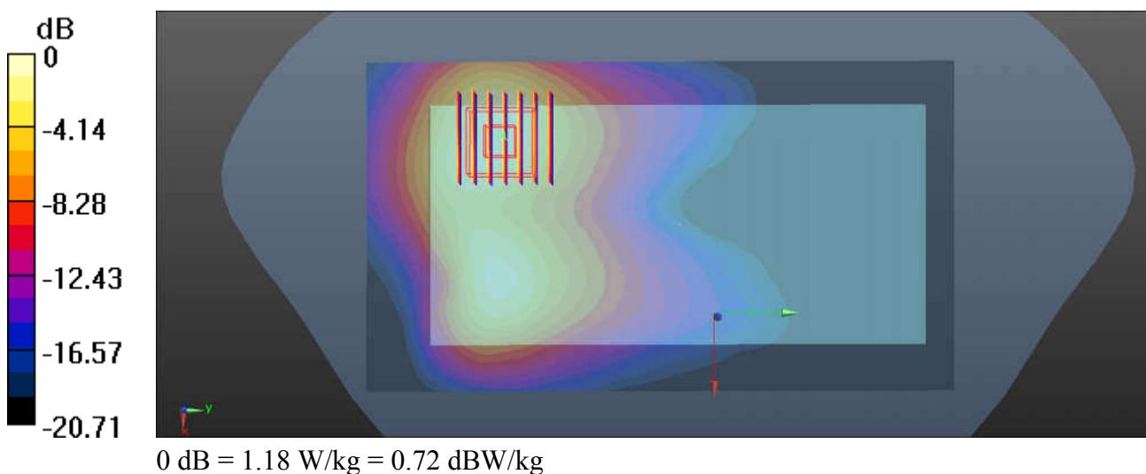
**44\_WLAN2.4GHz\_802.11b 1Mbps\_Top Side\_10mm\_Ch1\_Ant 1**
