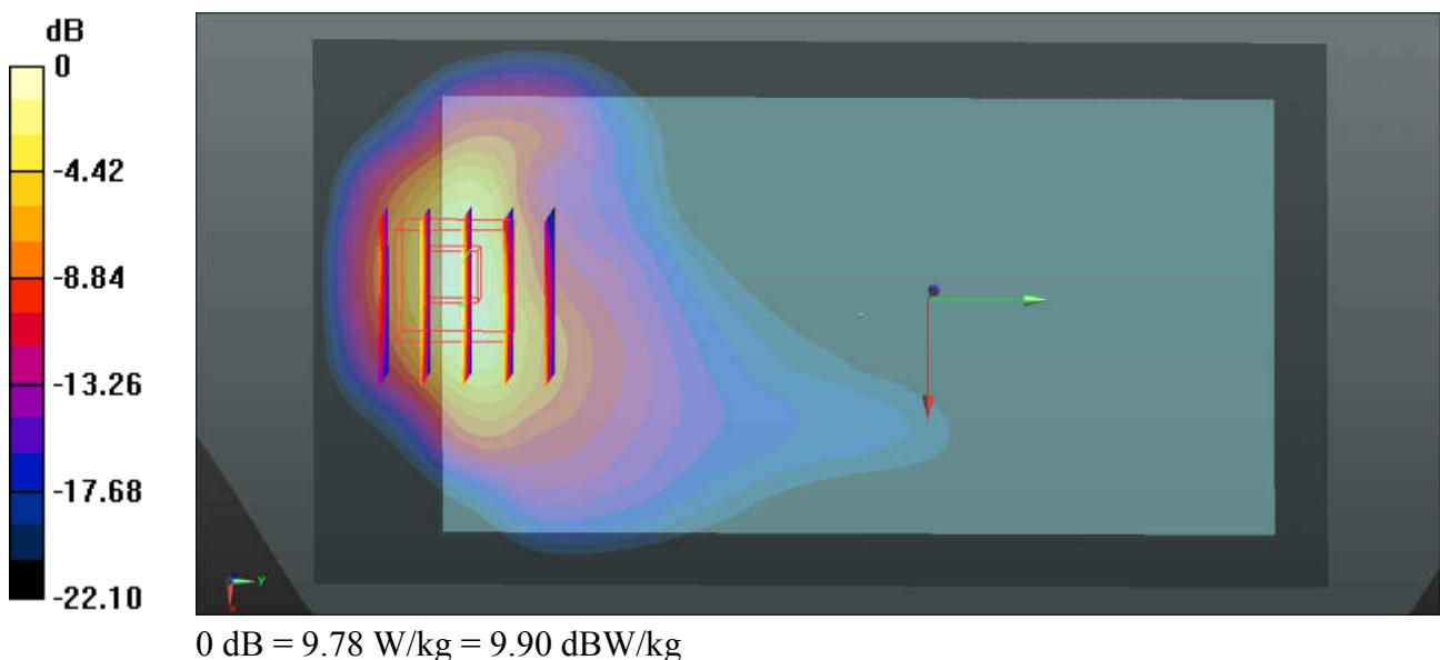
**77\_LTE Band 25\_20M\_QPSK\_1RB\_0Offset\_Back\_0mm\_Ch26140**
