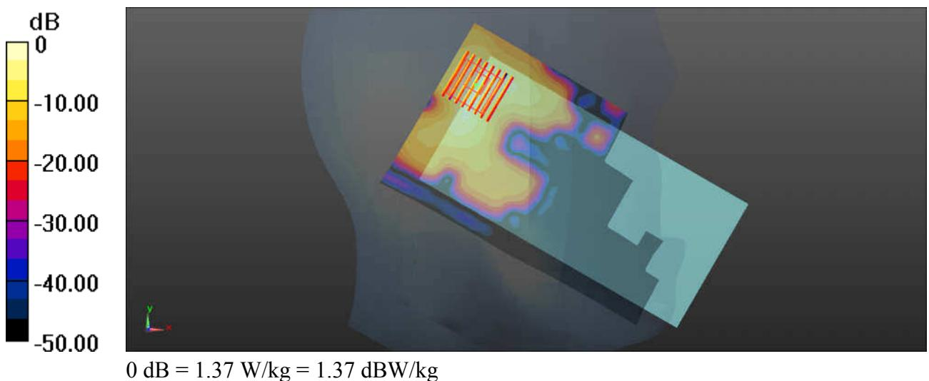
**20\_WLAN5.3GHz\_802.11a 6Mbps\_Left Cheek\_0mm\_Ch52\_Ant 2**
