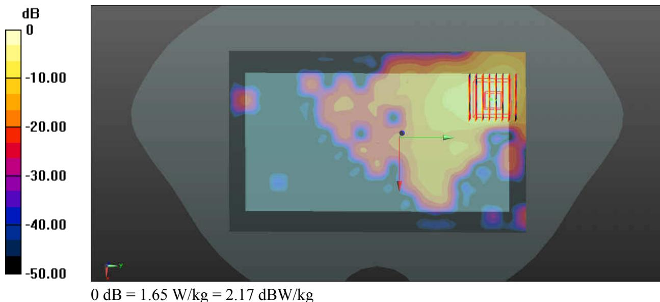
**66\_WLAN5.3GHz\_802.11a 6Mbps\_Back\_10mm\_Ch56\_Ant 2**
