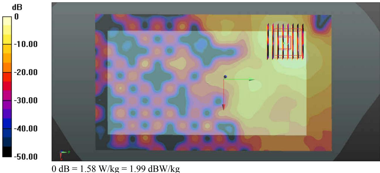
**52\_WLAN5.8GHz\_802.11n-HT20 MCS0\_Back\_10mm\_Ch165\_Ant 1+2**
