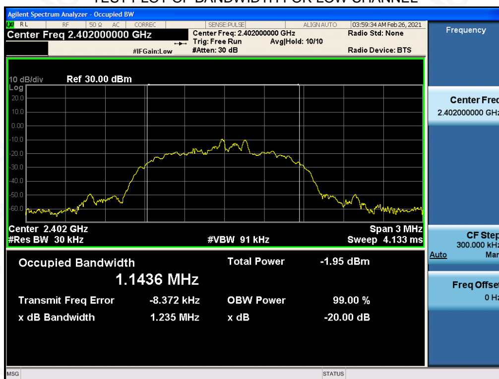
TEST PLOT OF BANDWIDTH FOR LOW CHANNEL
