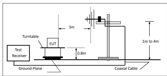
(c) For radiated emissions above 1000MHz
