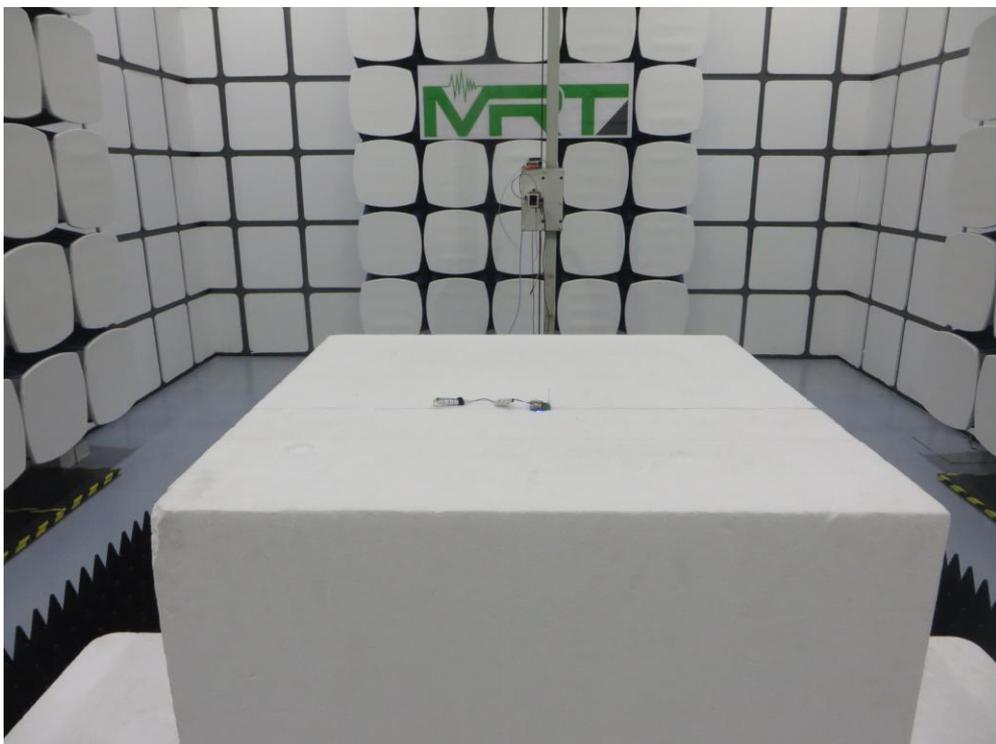
Description: Zoom-in Radiated Emission Test Setup
