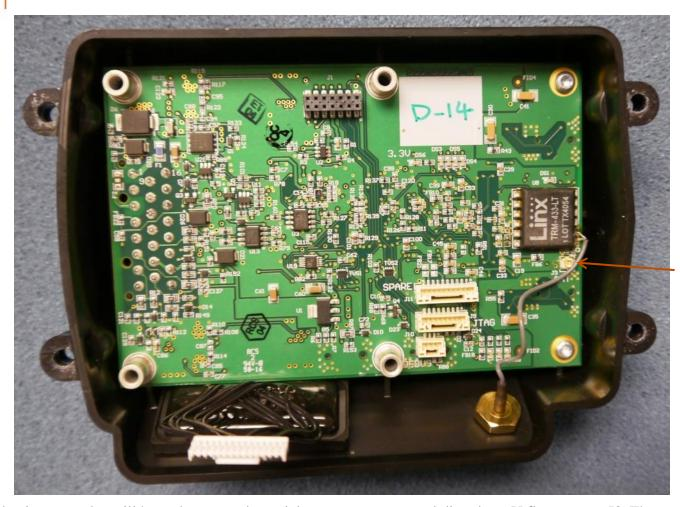
Note: Productions samples will have the external coaxial connector connected directly to U.fl connector J3. The tested sample had a faulty connector that had to be bypassed for testing. This change did not bypass any components or affect the RF output power delivered to the antenna.
