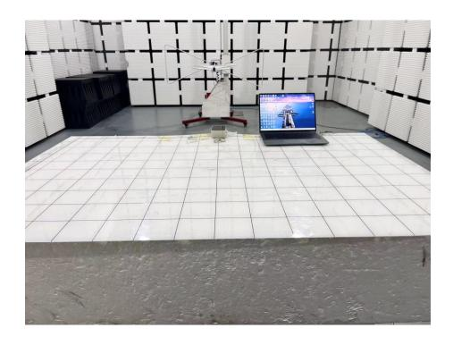
Set-up for Radiated Spurious Emission, Above 1GHz
