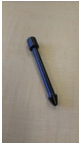
Fig. 16.2: Spindle to hold printer paper
