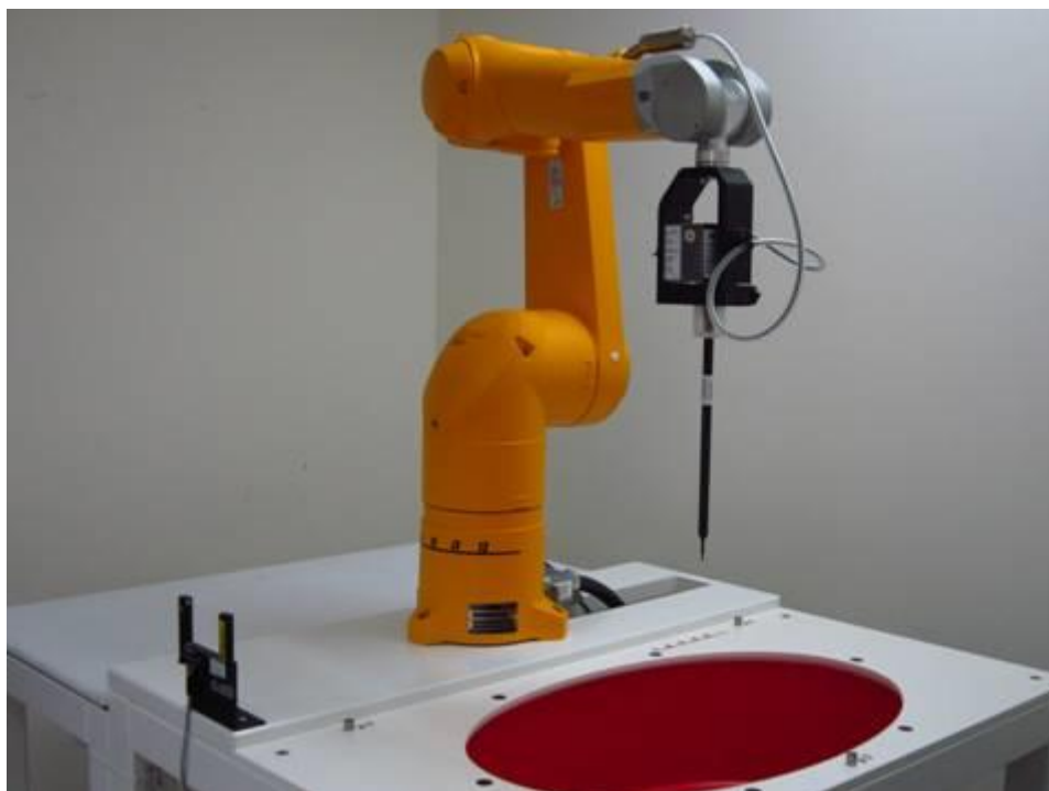
Fig.1 Photograph of the SAR measurement system
