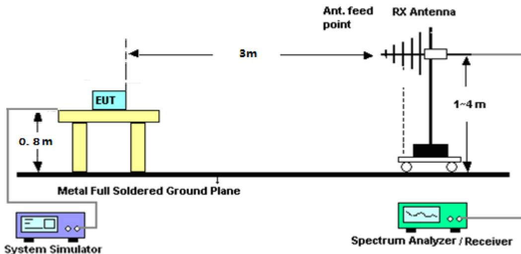
For radiated test from above 1GHz
