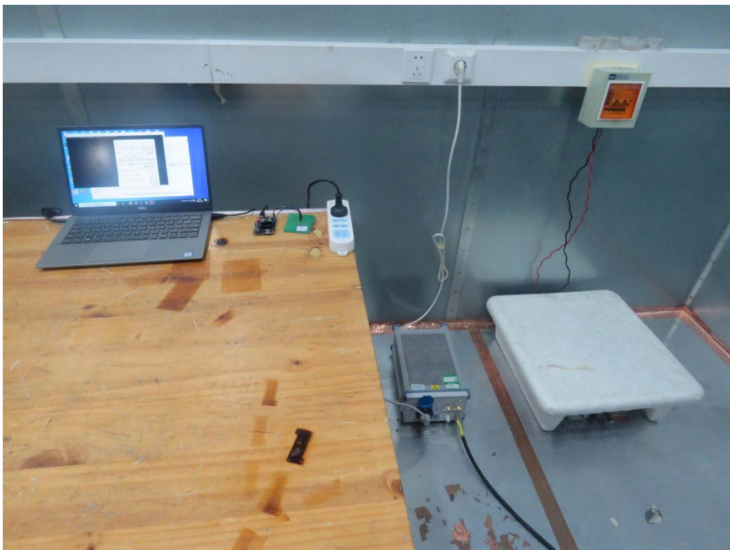
Picture 2 Conducted Emission Test Setup
