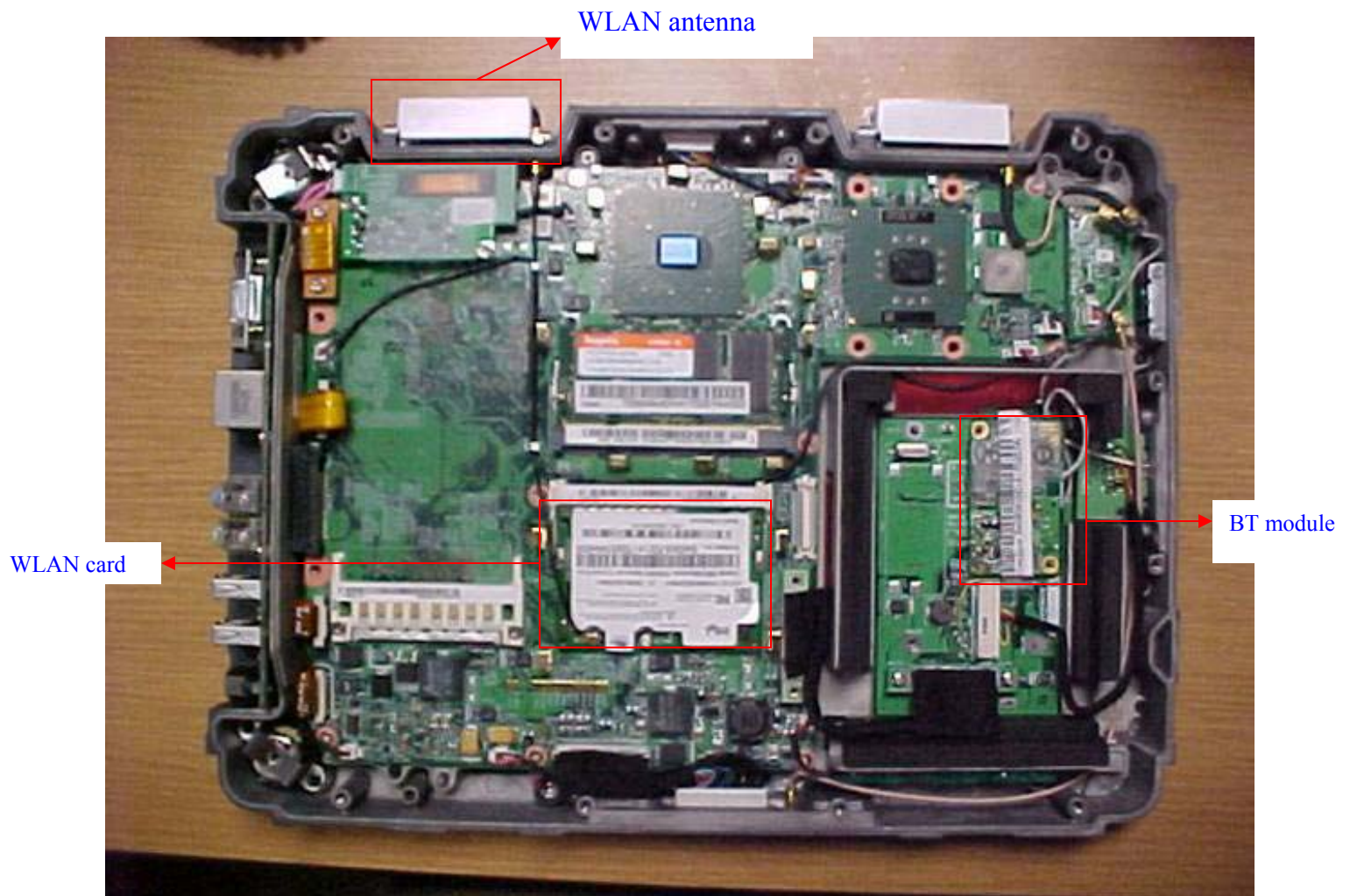
EUT – Internal view showing BT & WLAN module
