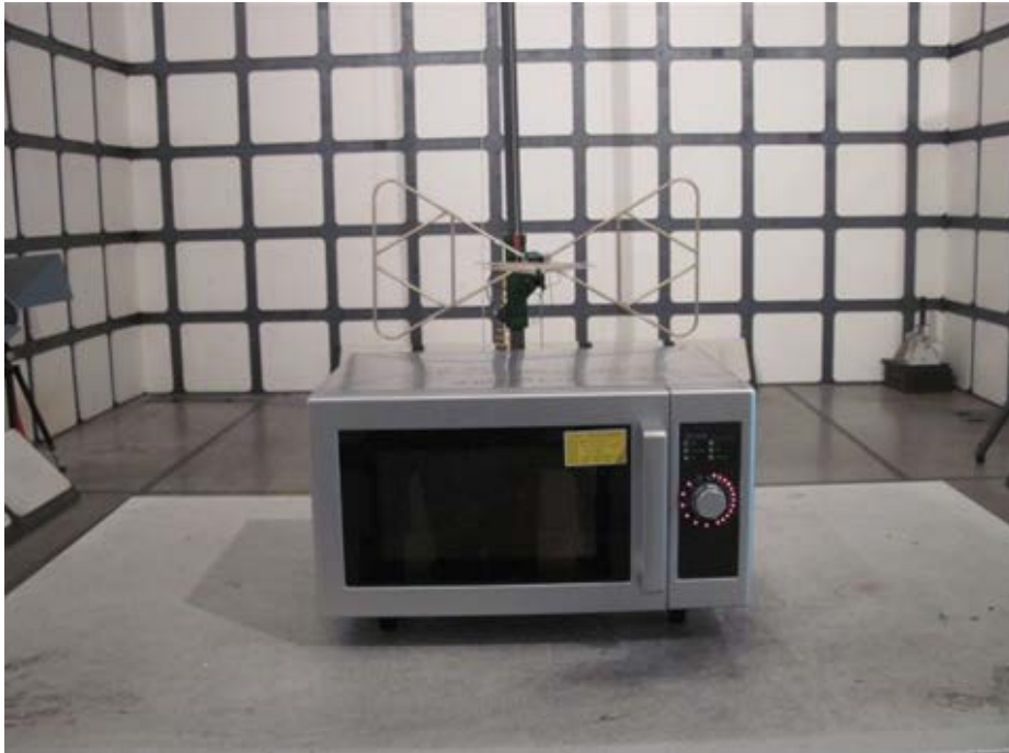
Radiated Emission Test Set-up (30-1000MHz): AM025FTR:
