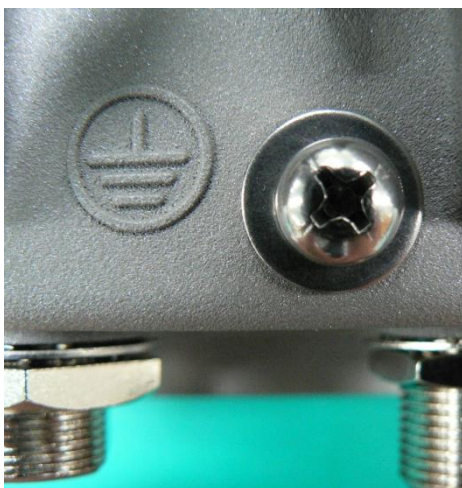
<Gemtek Small Cell Grounding Point Diagram>
