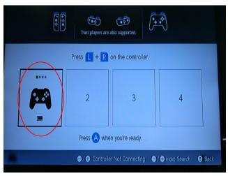
7. If there is no matching within 2 minutes, the controller will sleep automatically. Press Y+HOME on the wireless controller again to pair with the Switch console
