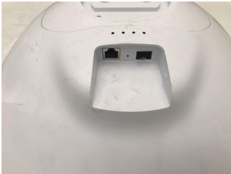
Photograph 7: Close Up of RJ45 Connector – Cover Removed
