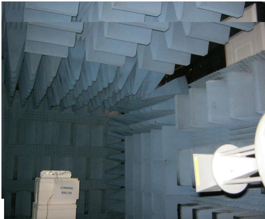
Figure 7. Radiated Emission Test
