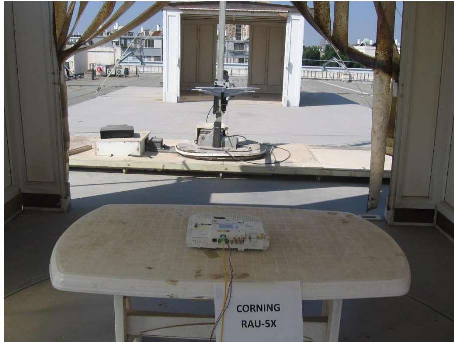
Figure 5. Radiated Emission Test
