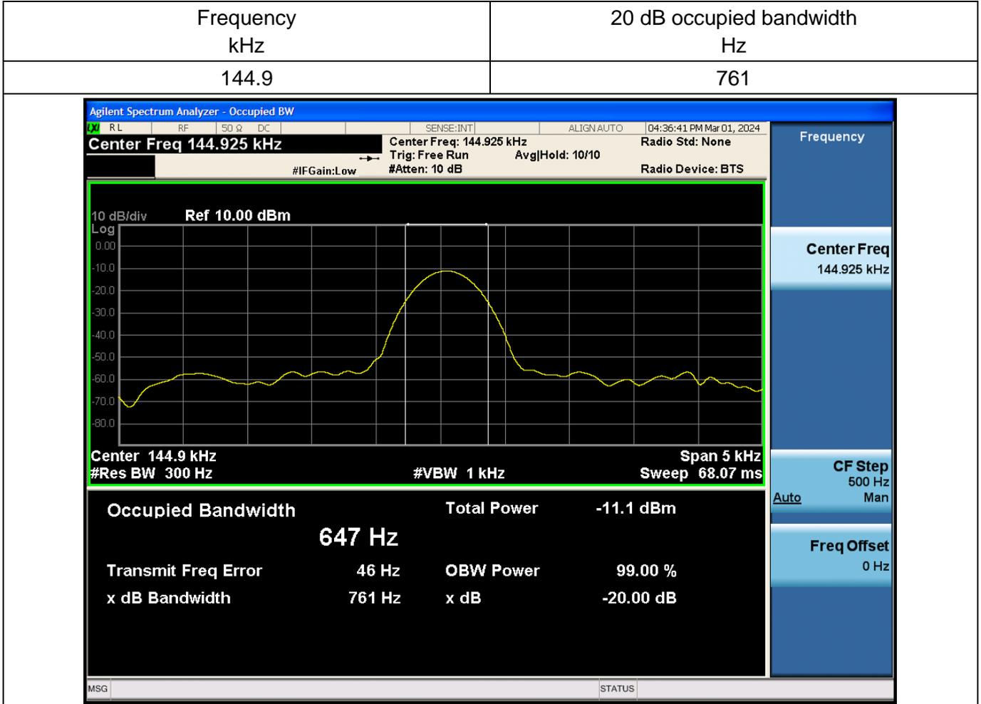
**Note:** Because the measured signal is CW-like, adjusting the RBW per C63.10 would not be practical since measurement bandwidth will always follow the RBW. The RBW is set to 300 Hz to perform the occupied bandwidth test.
