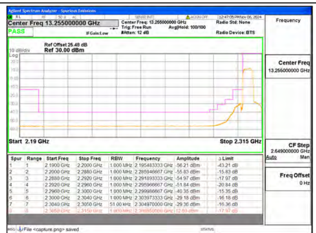
B30 / 5MHz / Low CH / QPSK / FULL RB
