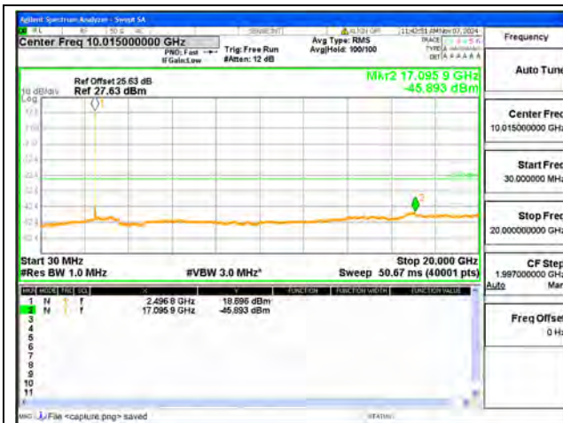
B41-30M-20G / 20MHz / Low CH / QPSK
