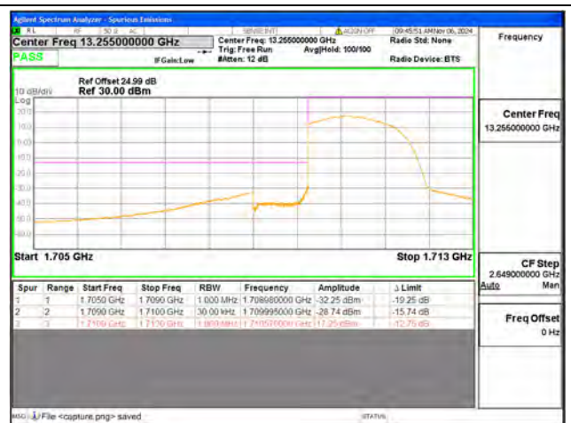
B4 / 1.4MHz / Low CH / QPSK / FULL RB
