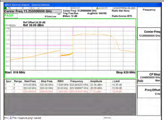
B26 / 3MHz / Low CH / QPSK / FULL RB
