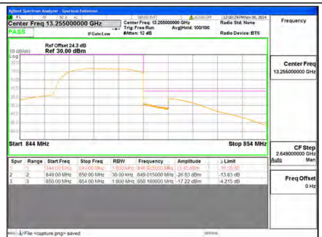
B26 / 3MHz / High CH / QPSK / FULL RB
