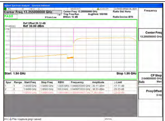
B25 / 10MHz / Low CH / QPSK / FULL RB
