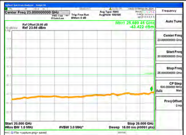
B7-20G-26G / 15MHz / Mid CH / QPSK
