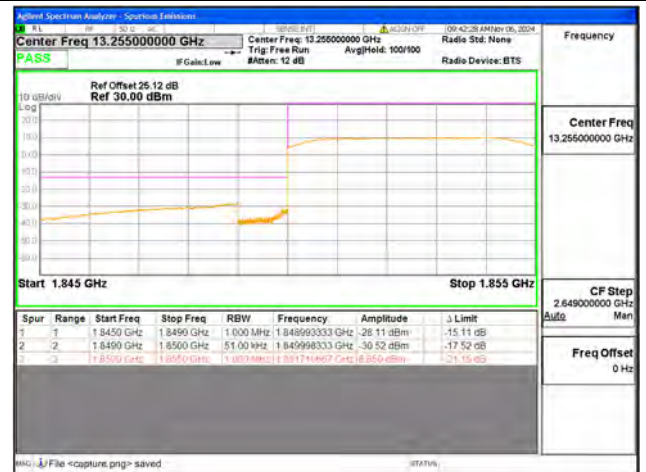
B2 / 5MHz / Low CH / QPSK / FULL RB
