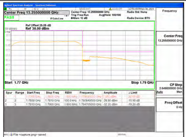
B66 / 10MHz / High CH / QPSK / FULL RB
