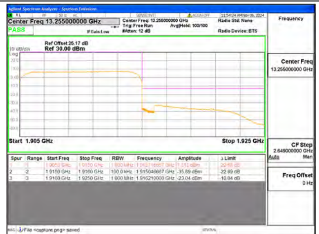
B25 / 10MHz / High CH / QPSK / FULL RB
