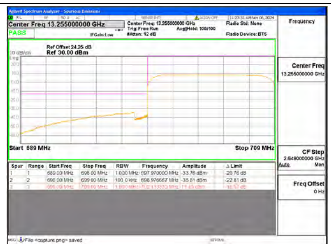
B12 / 10MHz / Low CH / QPSK / FULL RB
