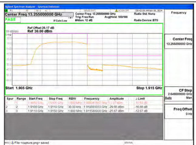
B2 / 3MHz / High CH / QPSK / FULL RB
