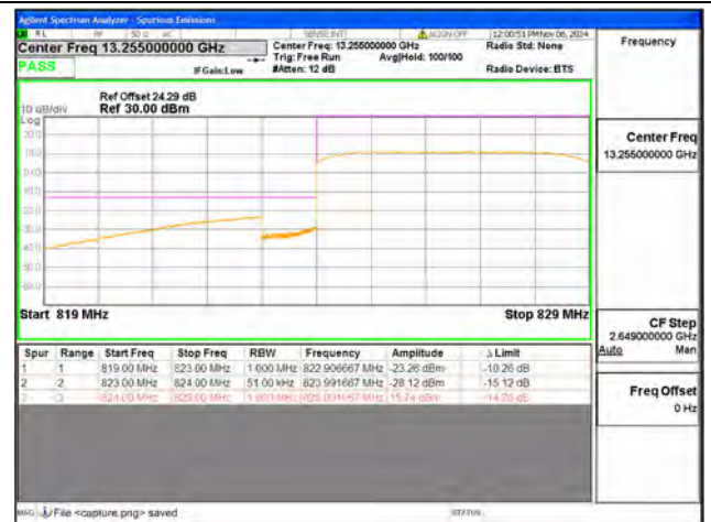
B26 / 5MHz / Low CH / QPSK / FULL RB
