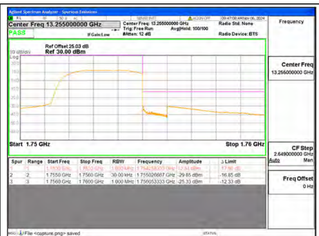
B4 / 3MHz / High CH / QPSK / FULL RB
