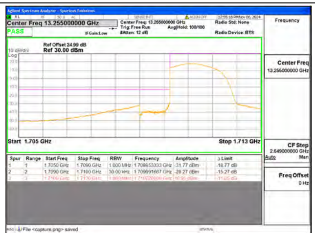
B66 / 1.4MHz / Low CH / QPSK / FULL RB
