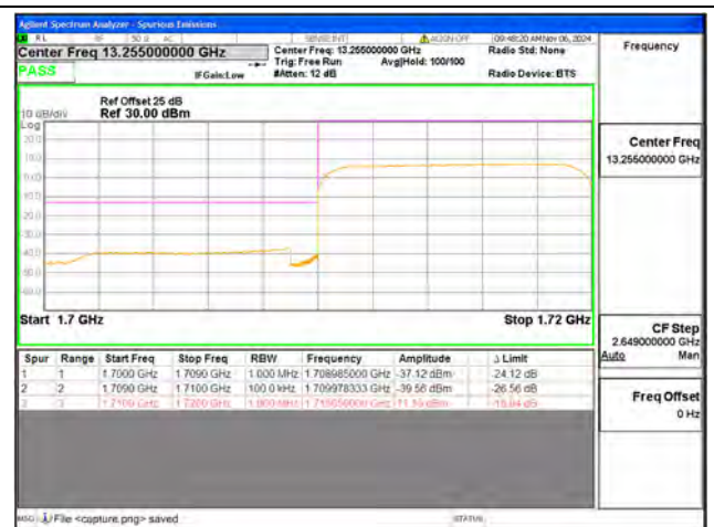
B4 / 10MHz / Low CH / QPSK / FULL RB
