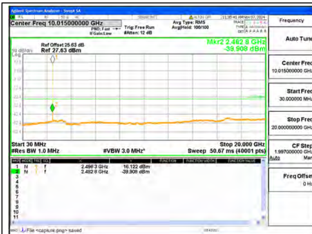
B41-30M-20G / 5MHz / Low CH / QPSK
