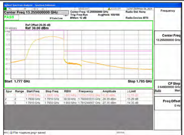
B66 / 1.4MHz / High CH / QPSK / FULL RB
