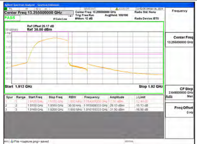
B25 / 1.4MHz / High CH / QPSK / FULL RB
