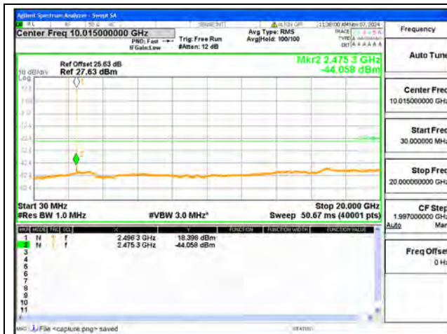
B41-30M-20G / 10MHz / Low CH / QPSK
