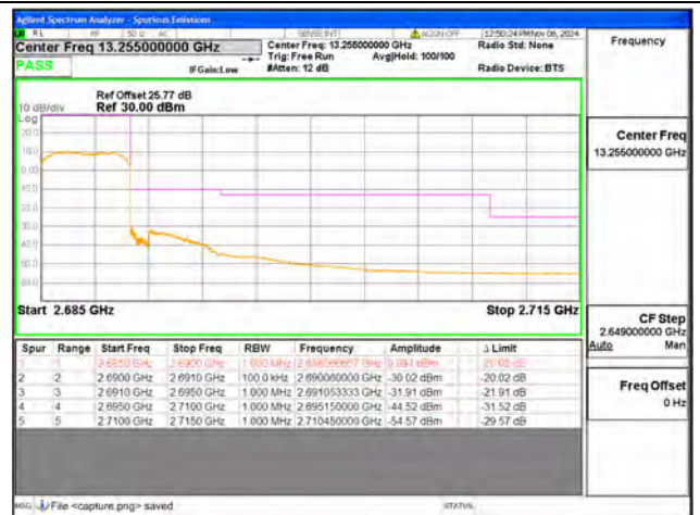
B41 / 5MHz / High CH / QPSK / FULL RB
