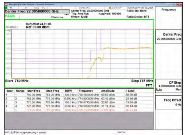
B13 / 10MHz / Low CH / QPSK / FULL RB
