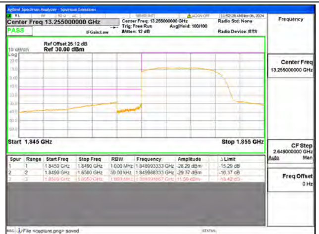
B25 / 3MHz / Low CH / QPSK / FULL RB
