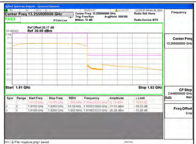
B25 / 5MHz / High CH / QPSK / FULL RB
