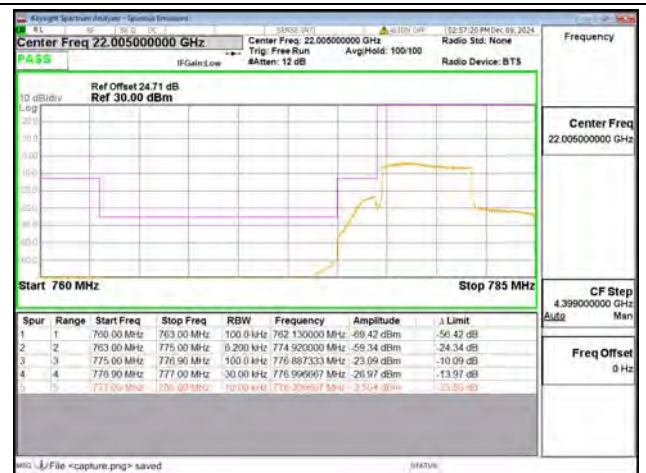
B13 / 5MHz / Low CH / QPSK / FULL RB
