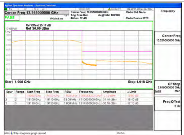
B2 / 5MHz / High CH / QPSK / FULL RB
