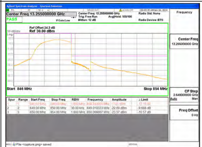
B5 / 1.4MHz / High CH / QPSK / FULL RB
