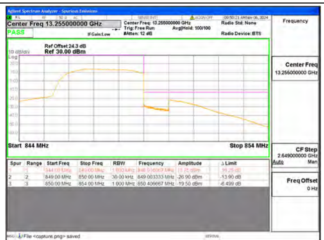
B5 / 3MHz / High CH / QPSK / FULL RB
