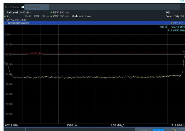
Plot 8-28. Conducted Spurious Emission Plot 652.1 MHz to 717.9 MHz (n26_1C_5M+n29_2C_5M+5M+n71_1C_20M_QPSK – Mid, Port0)
