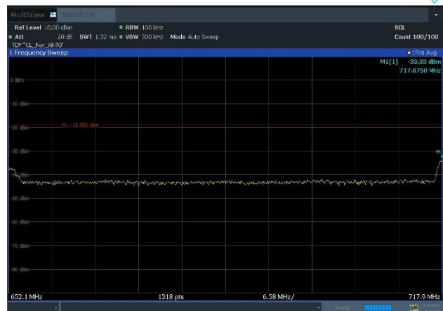
Plot 8-20. Conducted Spurious Emission Plot 652.1 MHz to 717.9 MHz (n26_1C_5M+n29_1C_5M+n71_1C_5M_QPSK – Mid, Port 0)
