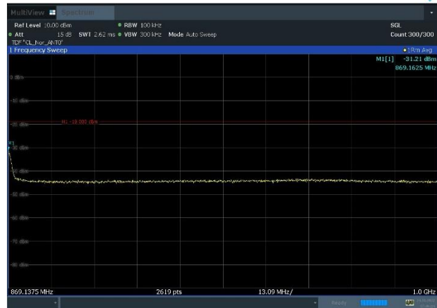
Plot 8-30. Conducted Spurious Emission Plot 869.1375 MHz to 1 GHz (n26_1C_5M+n29_2C_5M+5M+n71_1C_20M_QPSK – Mid, Port0)
