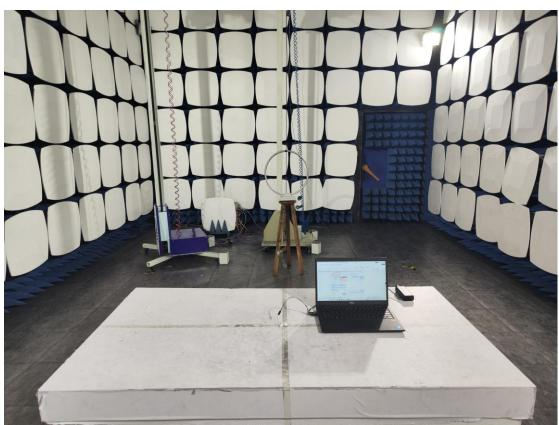
3. Radiated emission (9KHz-30MHz)
