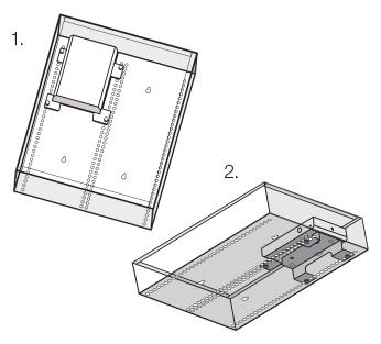
Shelf Mounting: The EL\_SC-100 has rubber feet to protect finished surfaces. Set the controller in a location that will allow you to properly manage connected wiring so that there is no tension on the connections.
