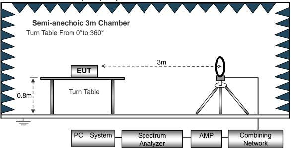
(B) Radiated Emission Test-Up Frequency 30MHz~1GHz
