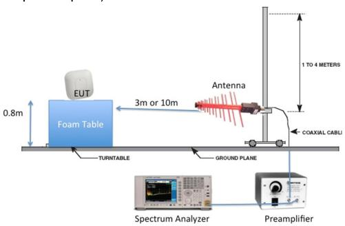
**Note:** The radiated spurious emissions test setup referenced to KDB789033 D02, v02r01, Section II (G)(3)(b)(i)), the EUT antenna ports were terminated with  $50\Omega$  loads.
