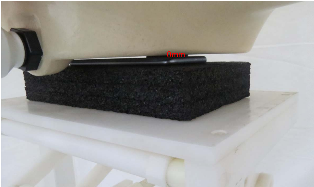
Picture 13: Back Side, the distance from handset to the bottom of the Phantom is 0mm
