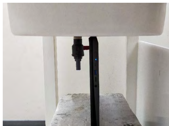
Fig.5 EUT Bottom side to flat phantom
