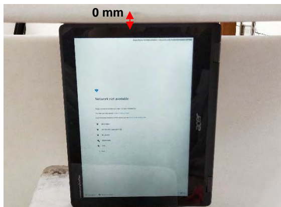
Fig.6 EUT Right side to flat phantom
