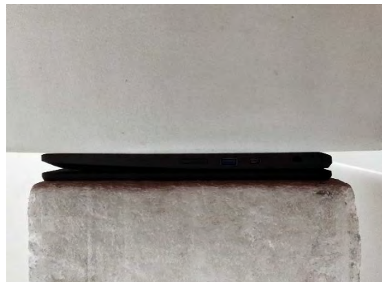
Fig.3 EUT Back side to flat phantom
