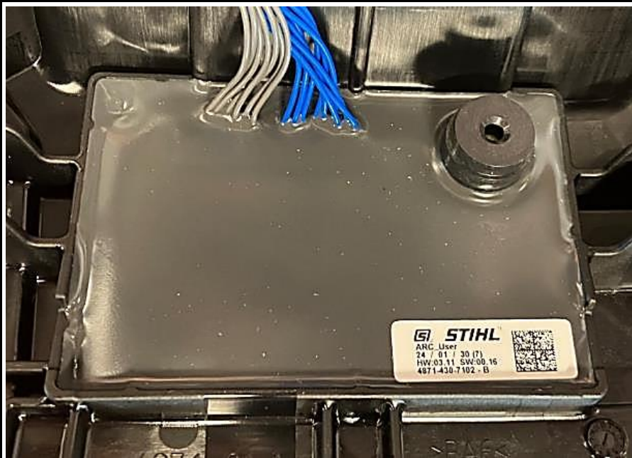
Module back side with potting - provided by customer
