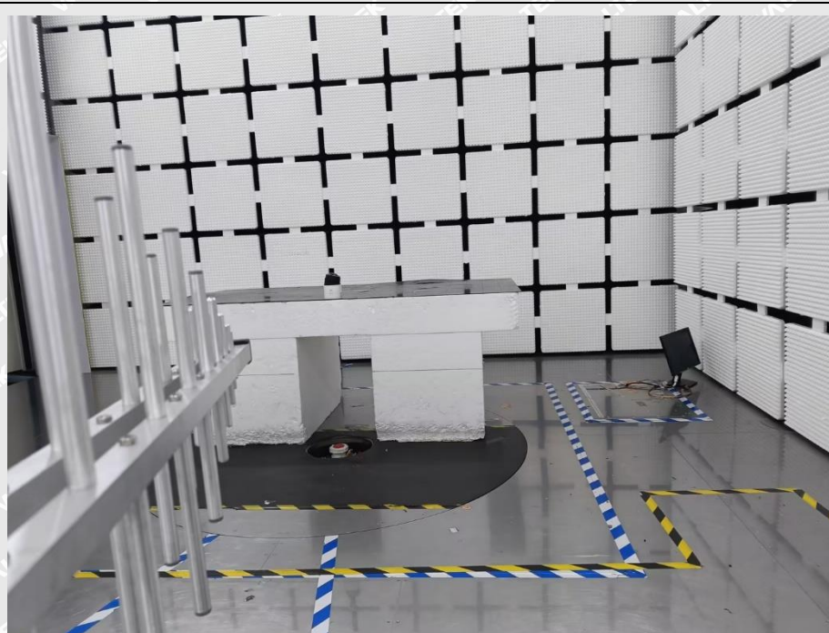
Radiation Emission Test Setup (30MHz to 1GHz)
