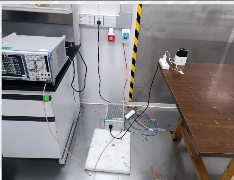
Conducted Emission Test Setup
