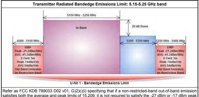
Refer as FCC KDB 789033 D02 v01, G)2)c)(i) specifying that if a non-restricted-band out-of-band emission satisfies both the average and peak limits of 15.209, it is not required to satisfy the -27 dBm or -17 dBm peak emission limit. Reason for change: to ensure that emission requirements in the non-restricted bands are not more stringent than those in the restricted bands.
