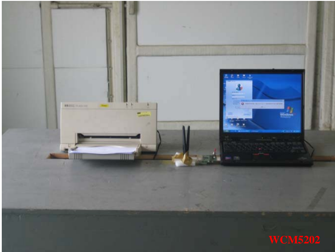
Photo 1: Radiated Emission Test Set-up
