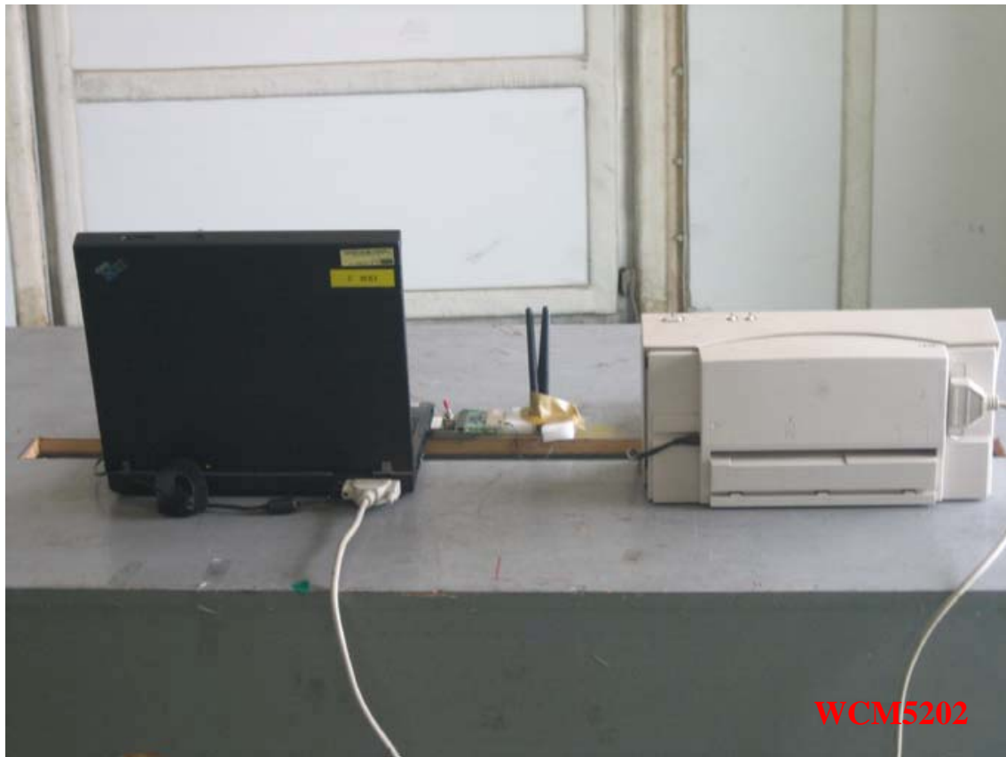
Photo 2: Radiated Emission Test Set-up
