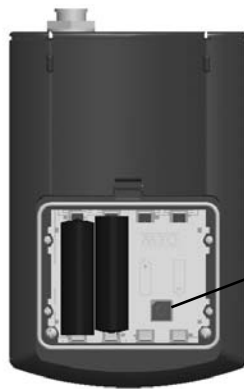
Figure 5. Rotary Switch in Battery Cradle
